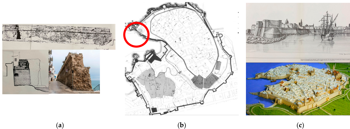
Figure 3. (a) The survey, section and view of the walls of the old gate, (b) the study on the construction phases of the walls (Capitanio D.) and (c) the iconography and model of the walls of Monopoli.
