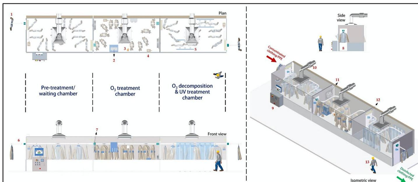
**Figure 3.** Automated ozone process for clothing and PPE disinfection showing the components of the system: (1) item of clothing or PPE; (2) ozone generator; (3) humidifier—dry fogger; (4) ozone sensor; (5) UVC tunnel; (6) conveyor; (7) transition system; (8) sliding door; (9) control panel; (10) extraction fan; (11) circulation fan; (12) air curtain (13) worker. Although not represented, UVC exposure may occur in the waiting chamber (1) before actual ozone treatment.
