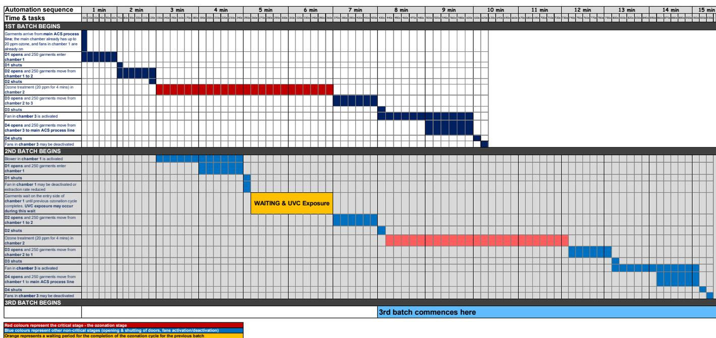
Figure 4. Process sequence of the automated ozonation system.
