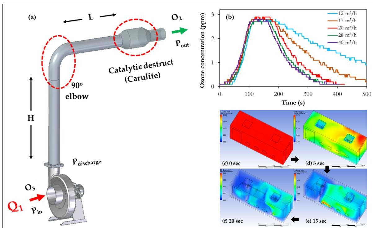
**Figure 7.** (a) Typical centrifugal fan system utilised for ozone gas removal; (b) analysis of ozone generation, stabilisation and decomposition using a lab-scale fan system [29]; application of CFD to analyse the removal rate of ozone gas in a chamber originally at 20 ppm.
