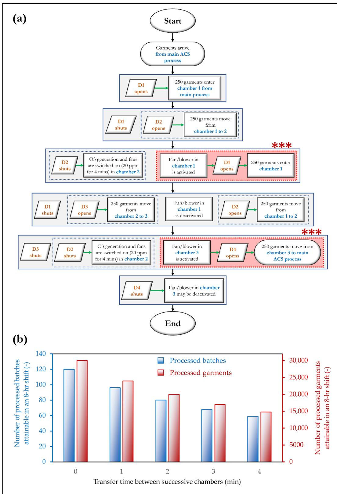
**Figure 5.** (a) Flowchart of the process sequence, with critical stages highlighted in red, and with an asterisk; (b) impact of garment transfer time on the throughput of the automated ozone decontamination system; ‘0’ represents an instantaneous transfer of the garments; although this is not possible in practice, it is useful for troubleshooting discrete event simulations of the process.
