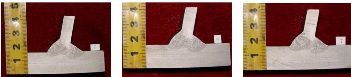
**Figure 5.** Macro-section of double-sided full-penetration rib-to-deck welded joints.
