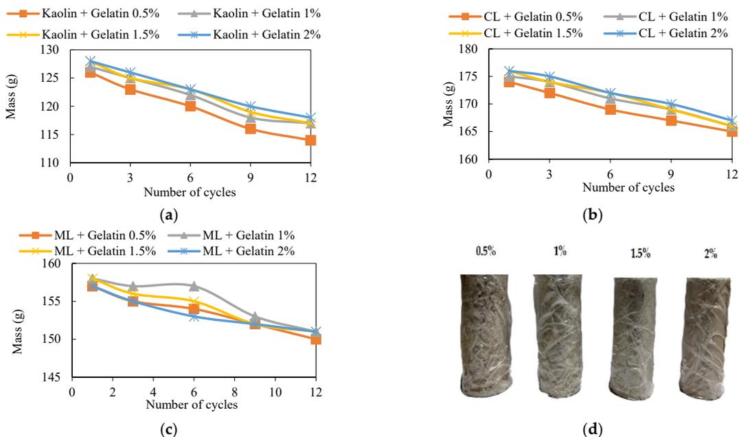
Figure 8. Durability test. (a) CH + Gelatin; (b) CL + Gelatin; (c) ML + Gelatin; (d) Durability specimens after 12 cycles.
