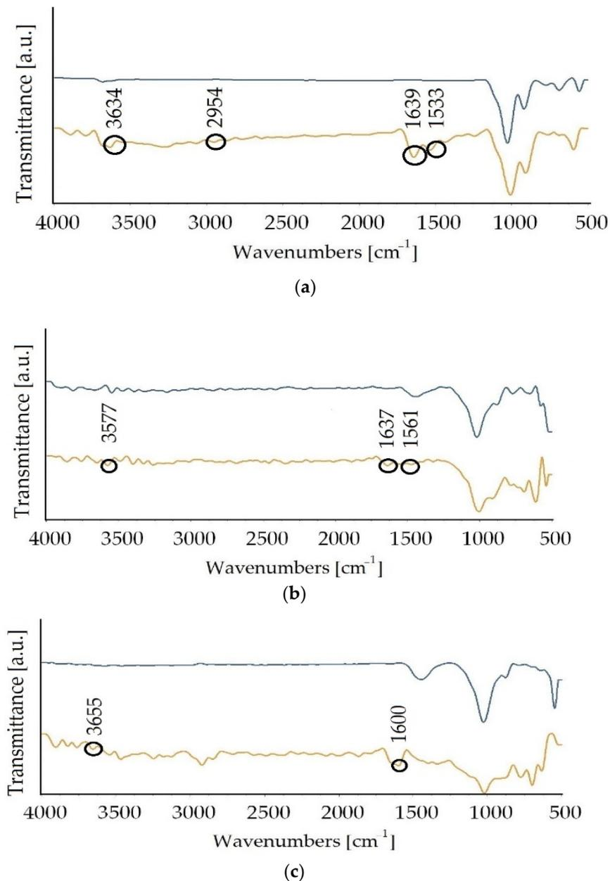
**Figure 9.** FTIR of Gelatin treated soils: (a) CH + Gelatin; (b) CL + Gelatin; (c) ML + Gelatin. Blue line represents soil. Orange colored line indicates gelatin stabilized soils.
