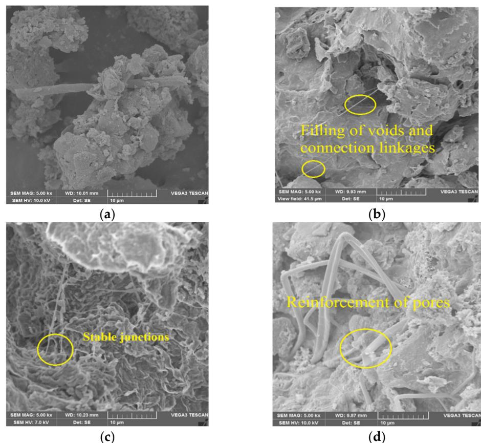
**Figure 10.** SEM of Gelatin treated soils: (a) Untreated CL; (b) Gelatin treated CH; (c) Gelatin treated CL; (d) Gelatin treated ML.
