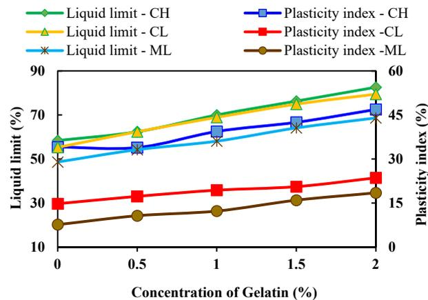
Figure 2. Liquid limit and plasticity index of gelatin-treated soils.
