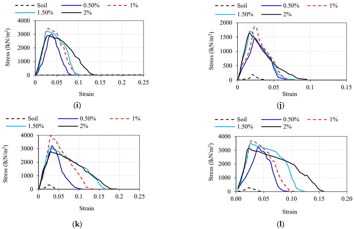
**Figure 5.** Stress-strain curves of UCS tests: (a) CH + Gelatin—2 h; (b) CL + Gelatin—2 h; (c) ML + Gelatin—2 h; (d) CH + Gelatin—3 days; (e) CL + Gelatin—3 days; (f) ML + Gelatin—3 days; (g) CH + Gelatin—7 days; (h) CL + Gelatin—7 days; (i) ML + Gelatin—7 days; (j) CH + Gelatin—28 days; (k) CL + Gelatin—28 days; (l) ML + Gelatin—28 days.
