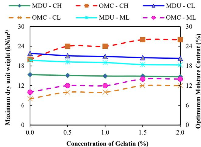
Figure 3. Compaction behavior of gelatin-treated soils.
