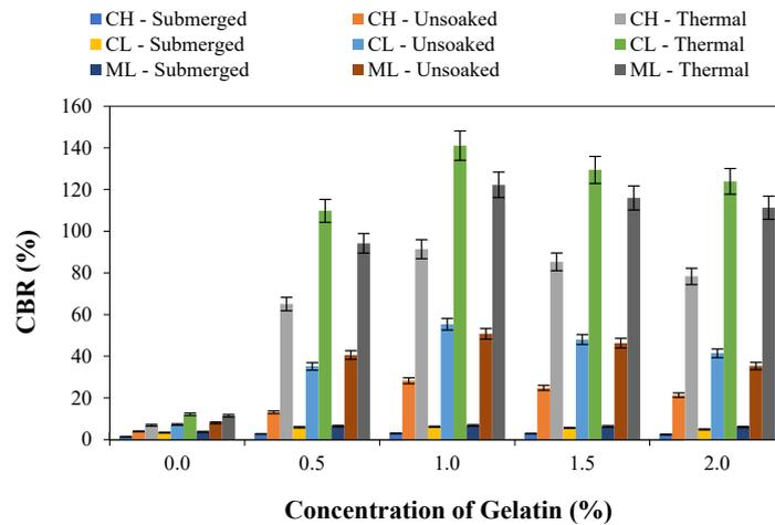
Figure 7. CBR of gelatin-treated soils.
