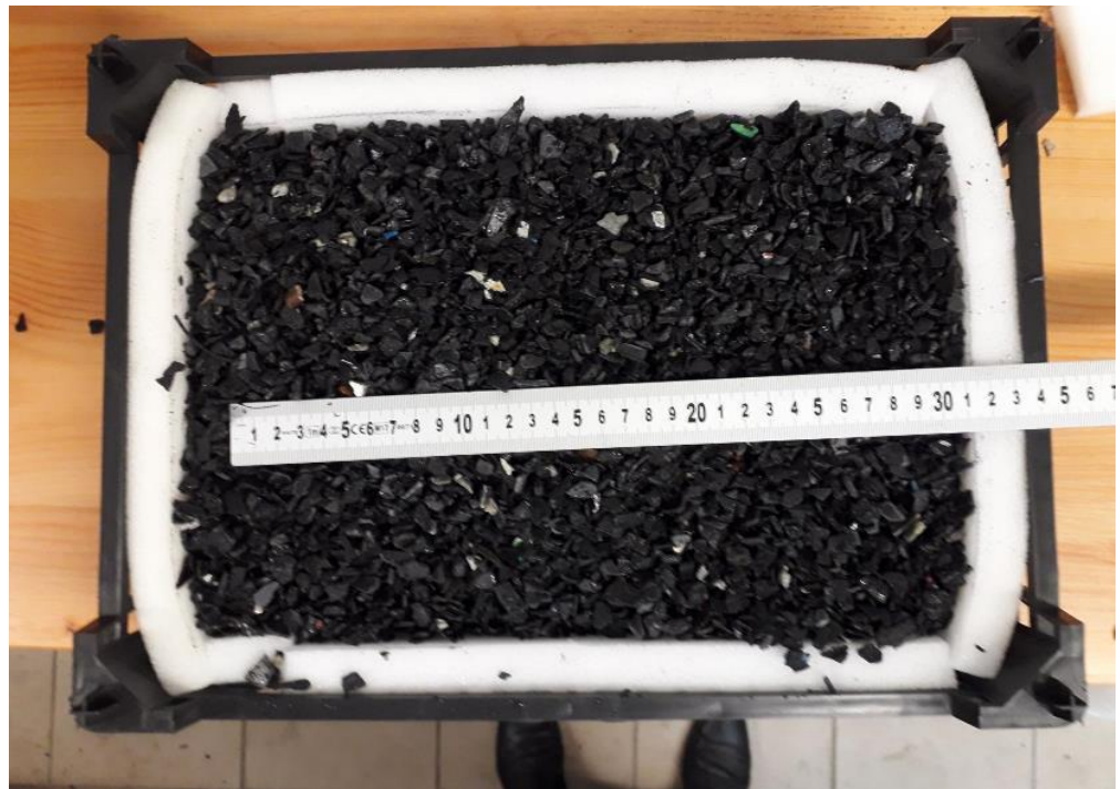
Figure A2. Box filled with the packing material—filter bed (variant with a uniform sponge base).
