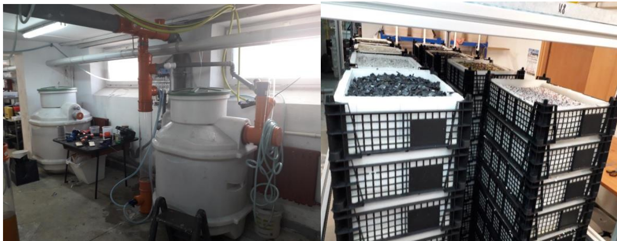
Figure A1. Test stand, primary septic tank—inflow of raw wastewater from the main building wastewater system and general view of the vertical flow filter.
