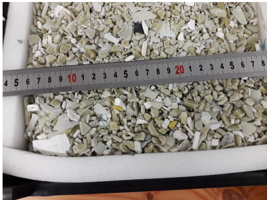
Figure A3. Shredded plastic (recycled ABS) used as the packing of the filter bed (shredded ABS from recycled WEEE recycling used as a filtering material).
