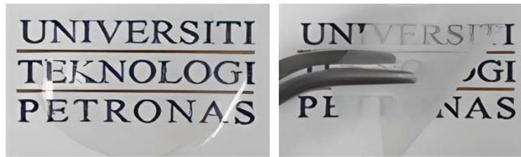
**Figure 1.** The physical appearance of the fabricated Pebax-1657/SAPO-34 CM.
