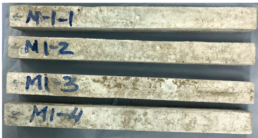
Figure 13. Geopolymer mixtures containing fresh BOFS aggregate submerged in water at 80^\circ\text{C} .
