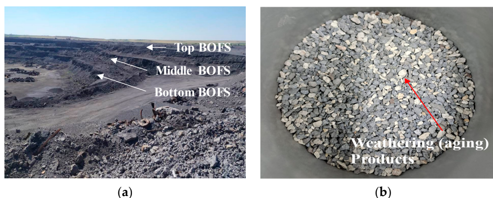
Figure 2. BOFS aggregate: (a) Field stockpiled BOFS with different ages. (b) Bottom BOFS.
