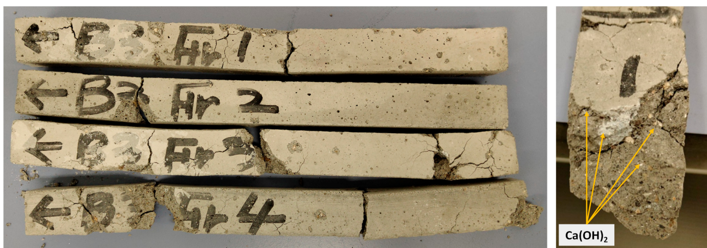
Figure 12. Normal OPC mixtures containing fresh BOFS aggregate submerged in water at 80 °C.
