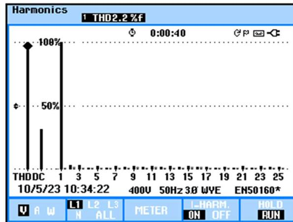
Figure 18. Experimental results of voltage THD analysis.
