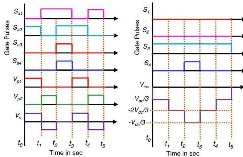
**Figure 7.** IMISO Z-source converter and SPFL inverter negative half-cycle switching patterns and output.
