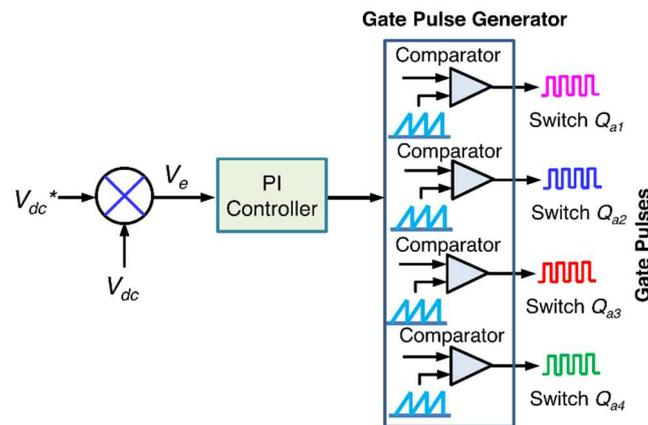
Figure 8. Voltage control of IMISO Z-source converter.
