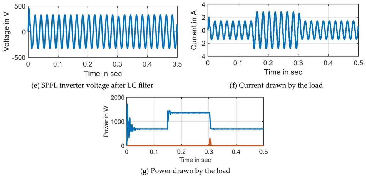
Figure 15. Simulation results of SPFL inverter and load.
