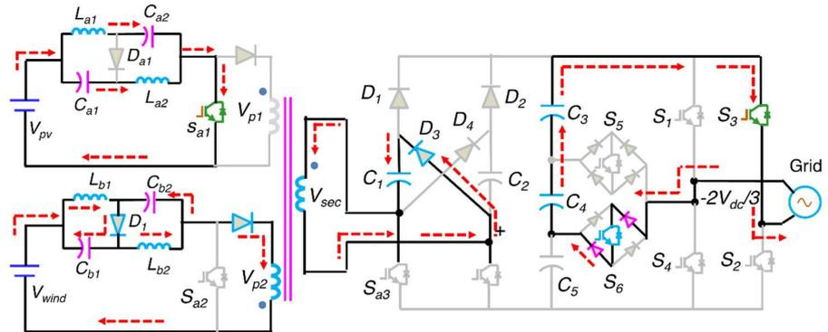
(b) Second interval of a negative half cycle
