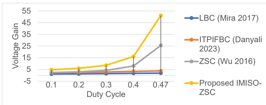
Figure 19. Comparison between the proposed IMISO Z-source converter and the standard converter [18–20].
