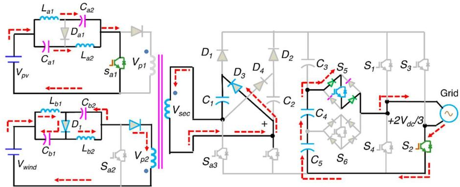
(b) Second interval of a positive half cycle
