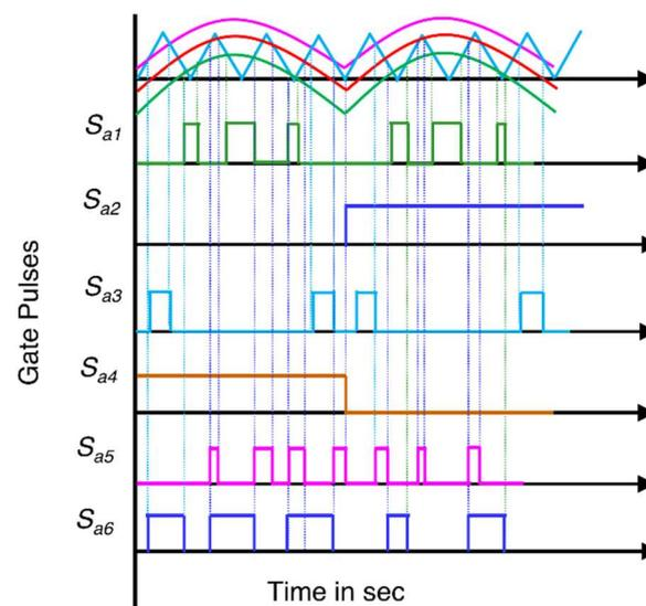
Figure 10. Gate pulse generation through hysteresis band.
