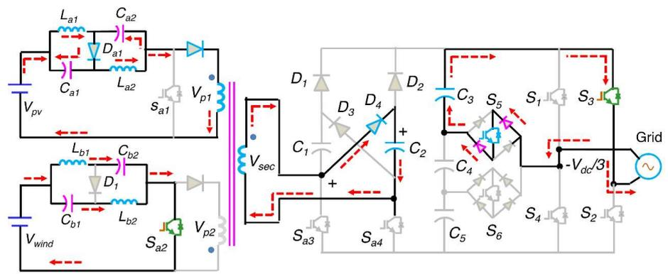
(a) First interval of a negative half cycle
