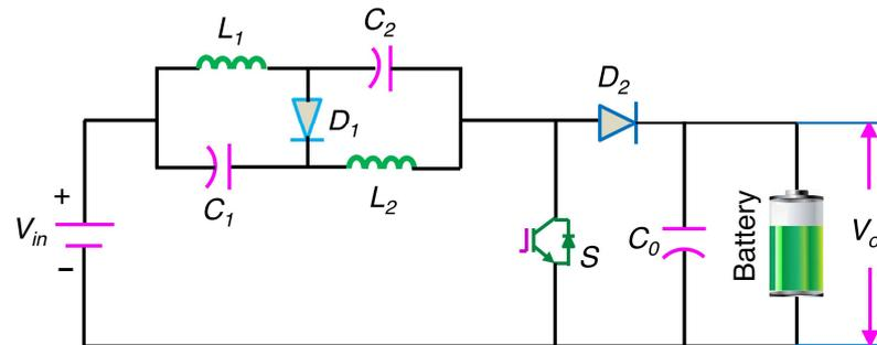
**Figure 1.** Impedance source converter using a conventional two-port configuration.
