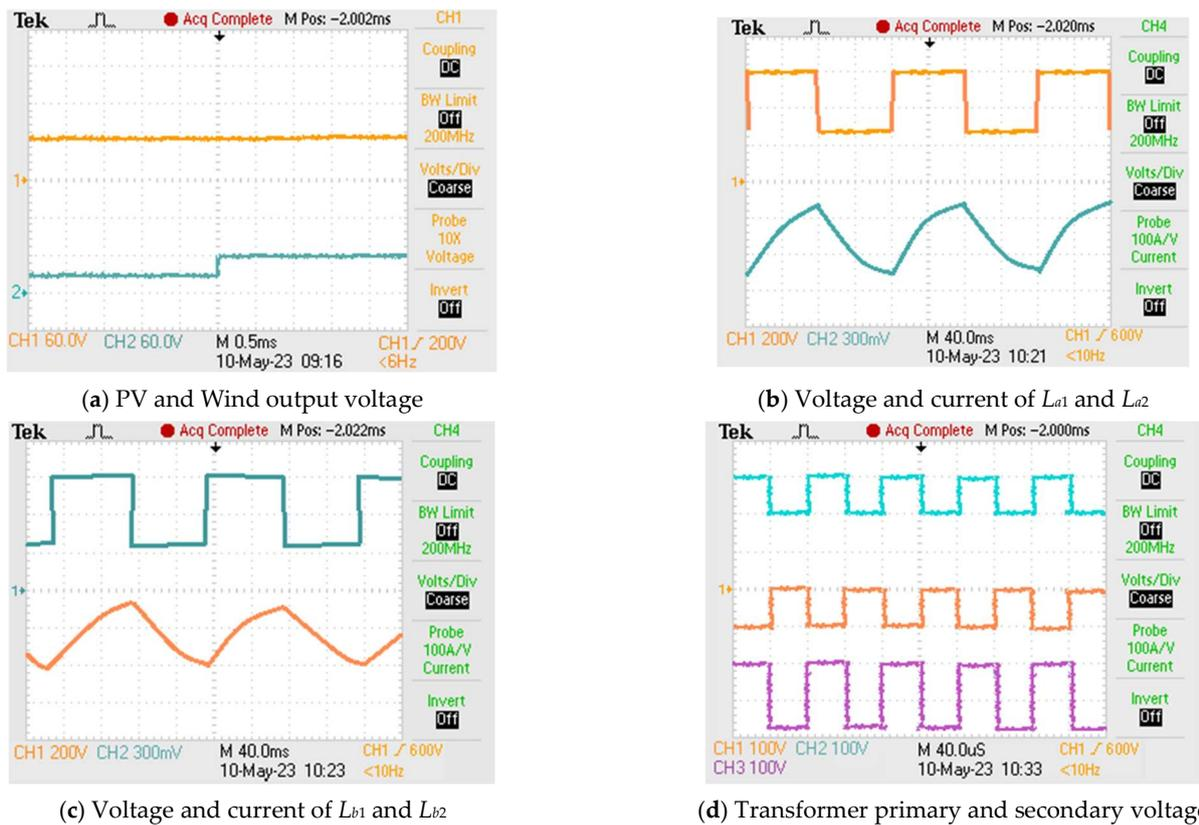
**Figure 13.** Experimental results of active and passive elements of IMISO-ZSC.
