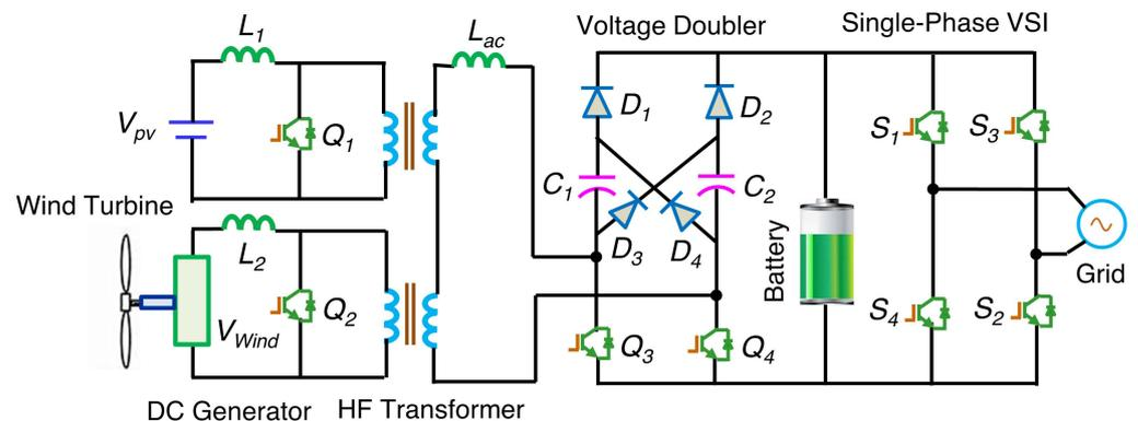
**Figure 2.** Conventional interleaved-boost full-bridge three-port converter.
