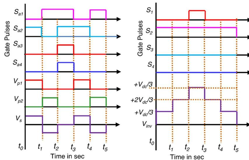
Figure 5. IMISO Z-source converter and SPFL inverter switching patterns and output.
