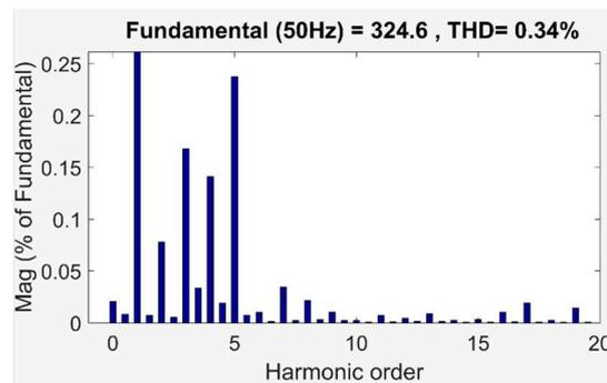
Figure 16. Simulation results of voltage THD analysis.
