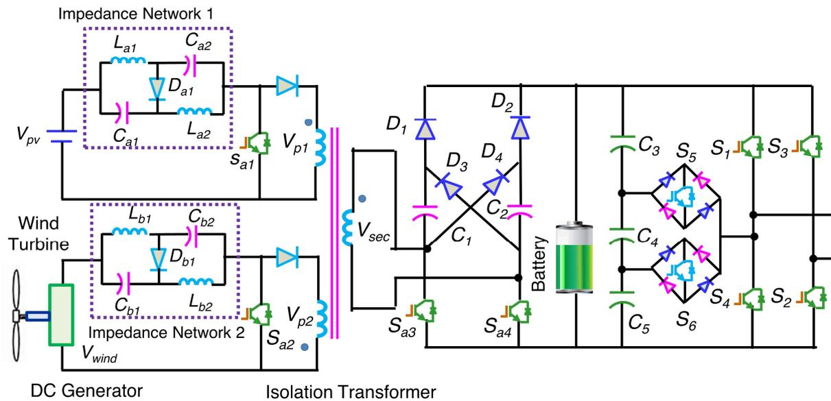
**Figure 3.** Proposed IMISO Z-source converter fed single-phase five-level (SPFL) inverter.
