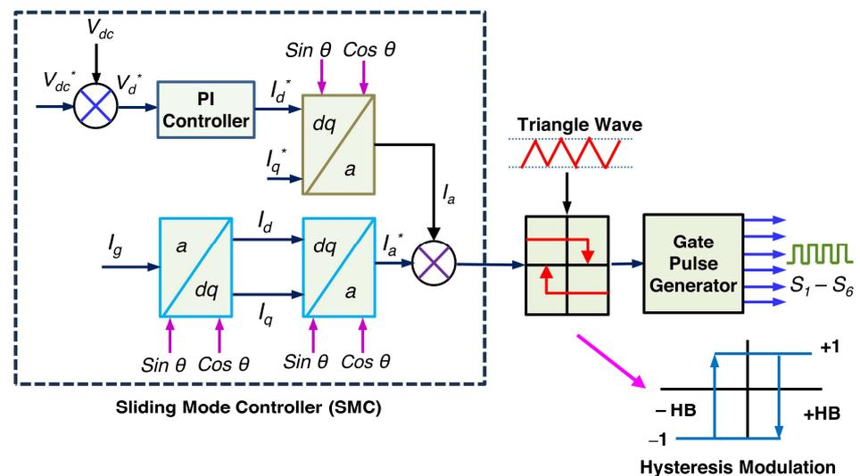
Figure 9. Sliding mode controller (SMC) with hysteresis modulation.
