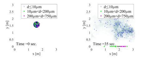
**Figure 2.** Flow of droplets over time; fluctuation level 0.05 m/s RMS for three different droplet sizes; own work with use of DNSLab [86].
