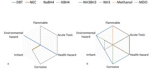
**Figure 1.** (a) Spiderweb of safety hazards of LOHCs (DBT and NEC) and borohydrides (NaBH<sub>4</sub> and KBH<sub>4</sub>); (b) Spiderweb of safety hazards of AB (NH<sub>3</sub>BH<sub>3</sub>), ammonia, methanol and MDO.
