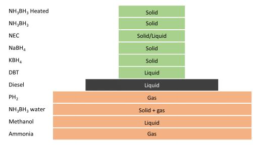
**Figure 4.** Qualitative comparison of hazards accompanied by future fuels and MDO relevant for the safety of crew and passengers. Here, only hazards are taken into account, no probabilities or resulting risks. Because of the different behaviors of substances due to their state, the state is taken into account.
