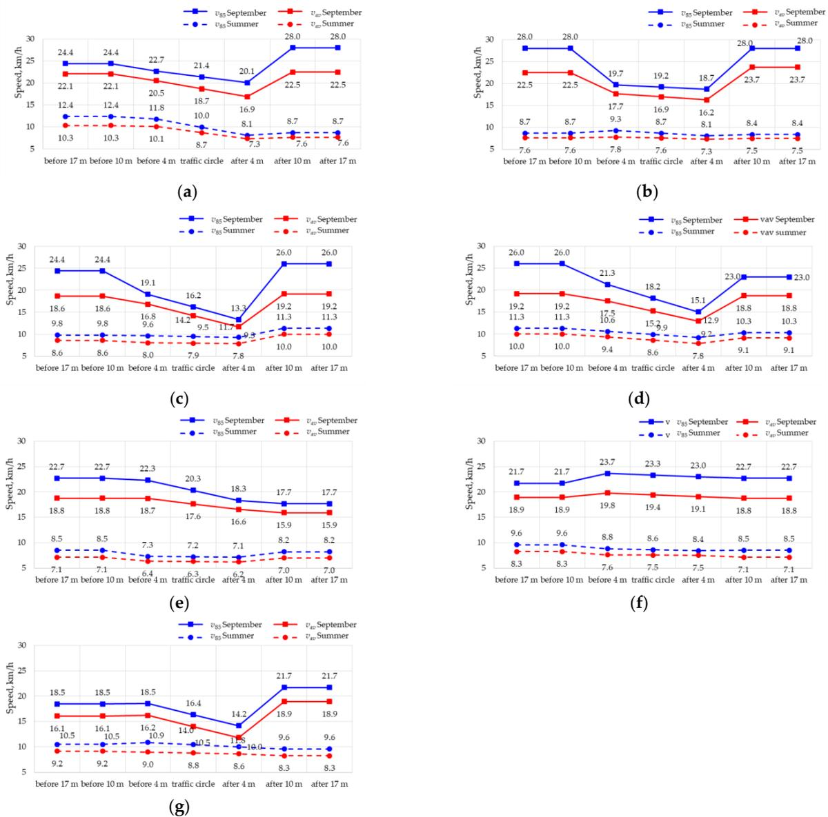
**Figure 17.** Traffic circle driving speed profiles: (a) No. 1— $\Delta h = 0.12$  m; (b) No. 2— $\Delta h = 0.09$  m; (c) No. 3— $\Delta h = 0.17$  m; (d) No. 4— $\Delta h = 0.16$  m; (e) No. 5— $\Delta h = 0.12$  m; (f) No. 6— $\Delta h = 0.08$  m; (g) No. 7— $\Delta h = 0.11$  m. Source: own work.
