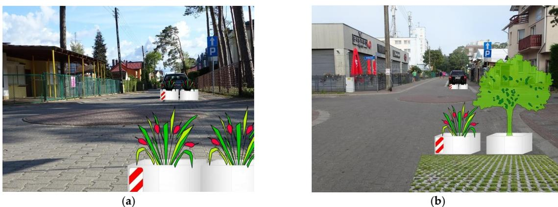
**Figure A1.** Visualization of the proposed traffic safety improvement measures using green infrastructure components suitable for home zone applications: (a) tree boxes with appropriately selected species used as side obstacles (greenery resistant to drought, frost, exhaust emissions); (b) side obstacles with appropriate grafted tree species. Source: own work.
