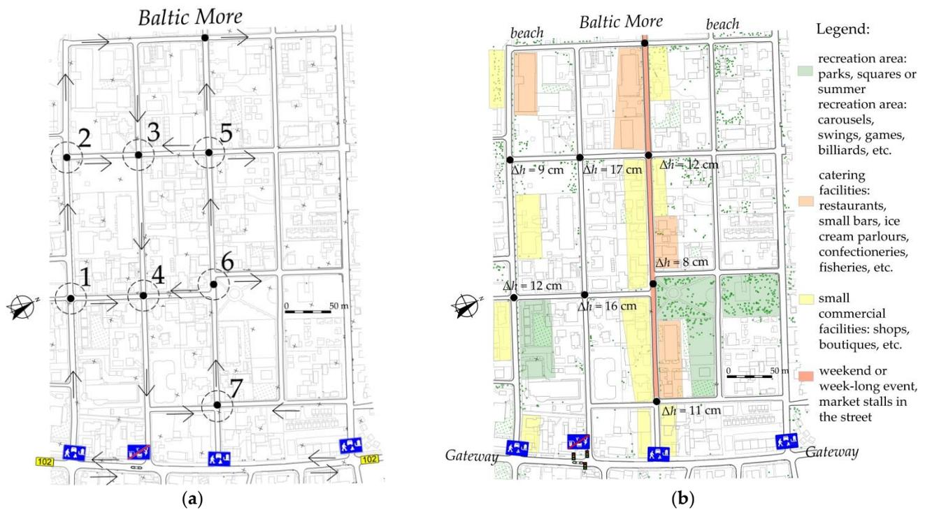
**Figure 6.** Study area details: (a) traffic circles' locations and numbering; (b) home zone divided into functional sub-areas. Source: own work.
