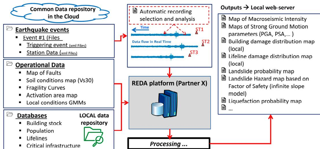
**Figure 1.** Rapid Earthquake Damage Assessment platform structure and Real-Time operational mode.
