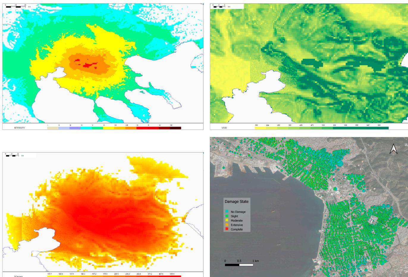
**Figure 8.** Seismic risk assessment of the building stock of Thessaloniki for the Volvi earthquake ( $M = 6.5$ , 1978), using the REDA platform: **(top left)** Intensity values in the greater area around the city of Thessaloniki; **(top right)** Vs30 values in a user defined grid; **(bottom left)** PGA values, in  $\text{cm/s}^2$ , **(bottom right)** damage state distribution estimates for the building stock in the metropolitan area of Thessaloniki.
