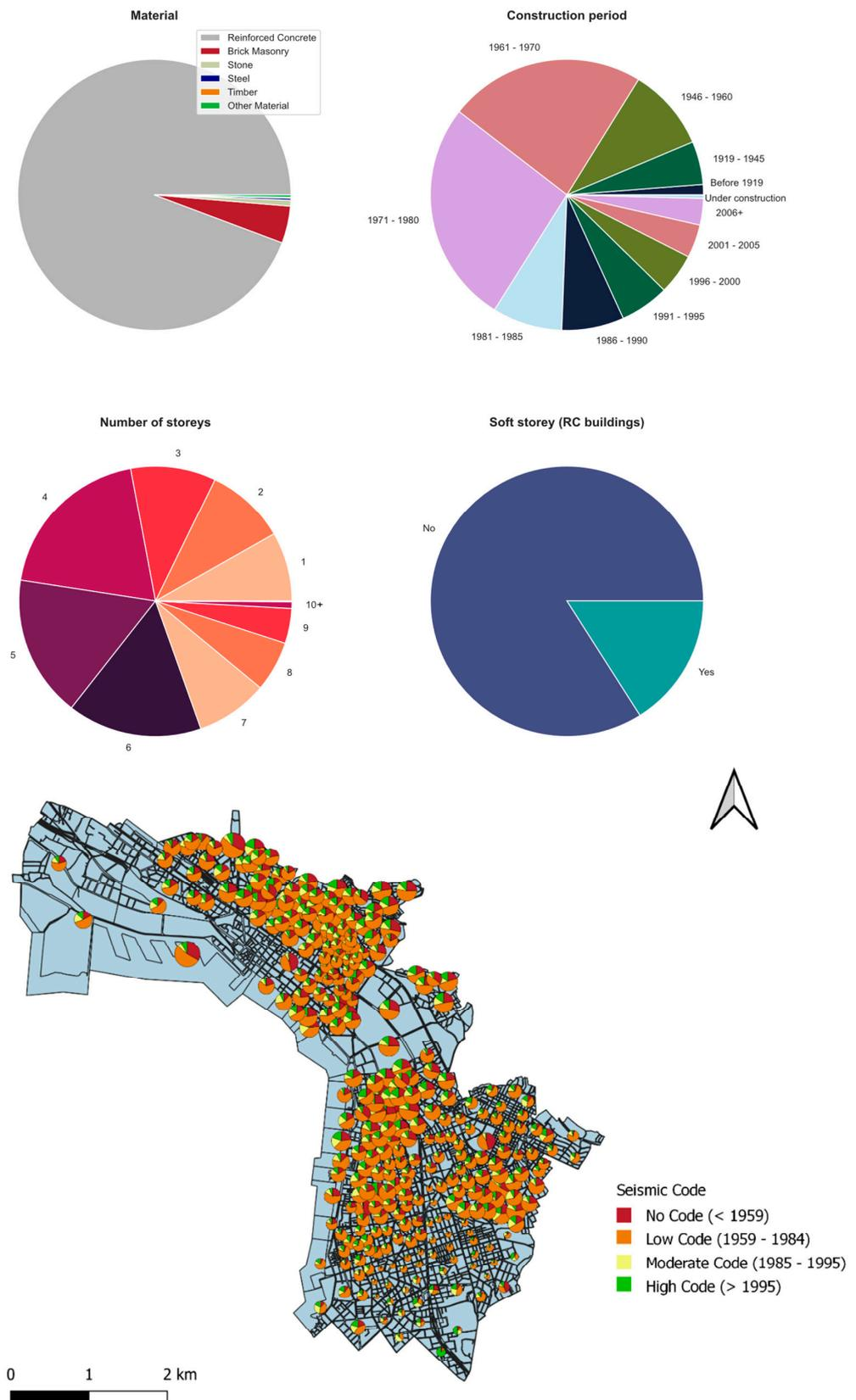
**Figure 7.** Main characteristics of the building stock in the Municipality of Thessaloniki (top); spatial distribution of the seismic design level in the building blocks of the city (bottom).
