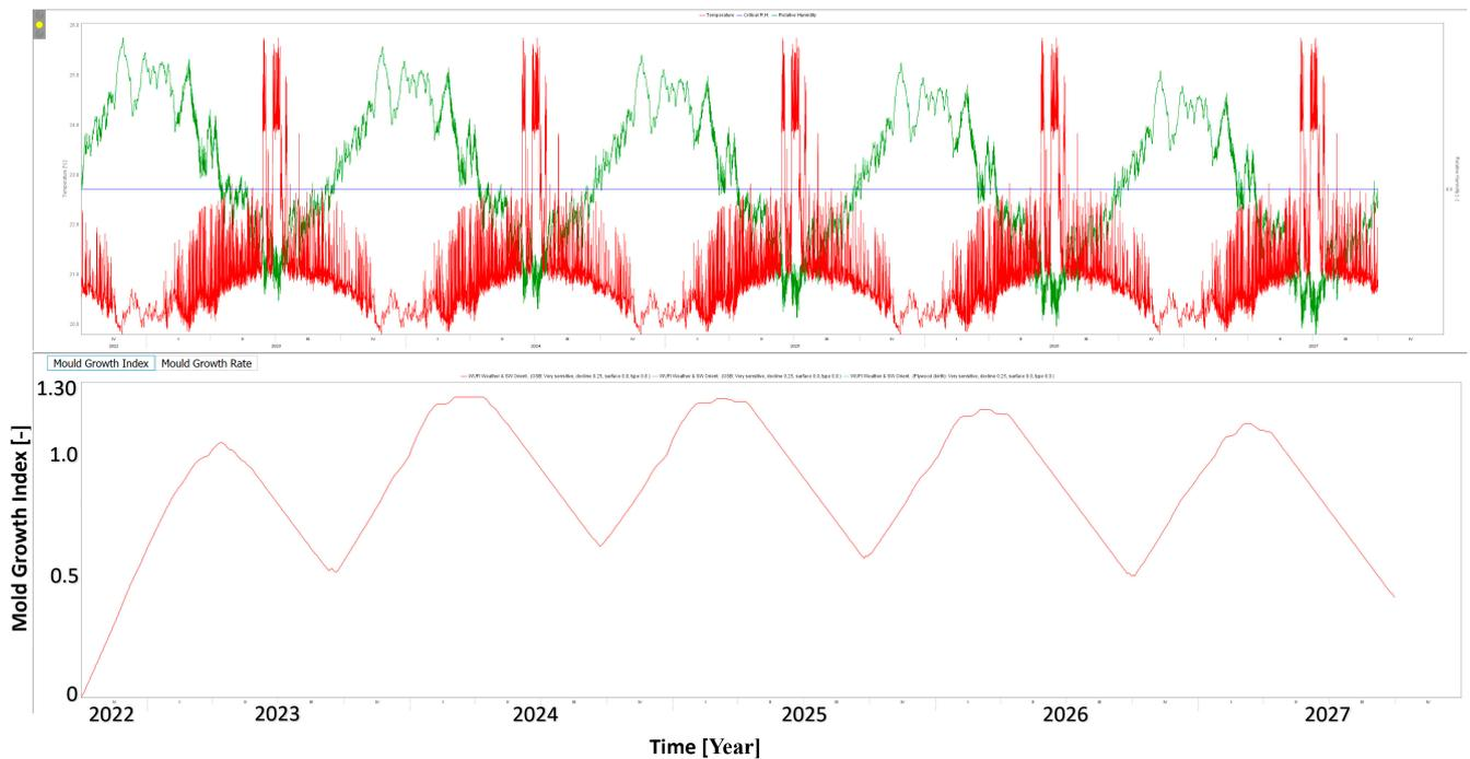
**Figure 13.** Mold growth index (MGI) for the inner plywood layer of the AHWs generated by WUFI® VTT—SW side.
