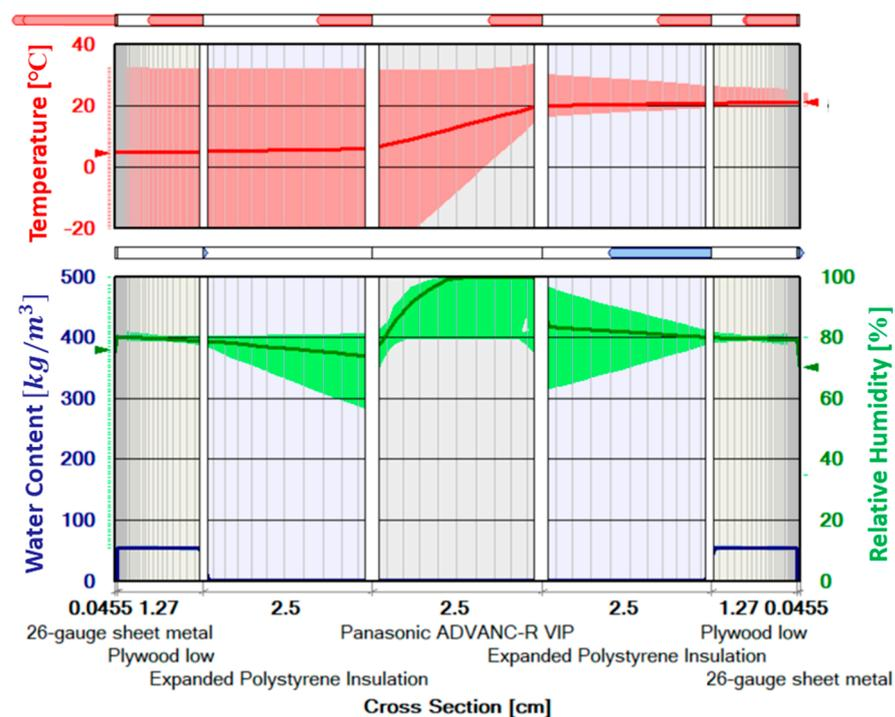
Figure 12. Mean climate profile of AHWs simulated on WUFI® over a five-year period—SW wall.
