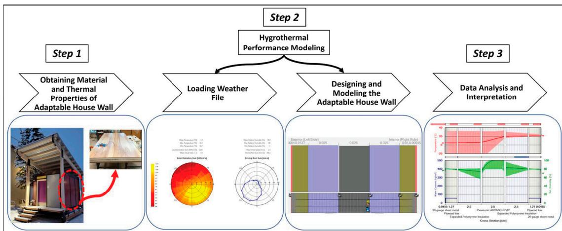
**Figure 1.** Methodology to evaluate the hygrothermal performance of the adaptable house wall in the extreme cold climate conditions of Alaska.
