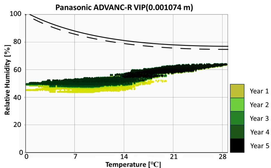
**Figure 11.** Isopleth graph at different intersections elements in the SW side of the AHW—Panasonic ADVANC-R vacuum insulation panel (VIP).
