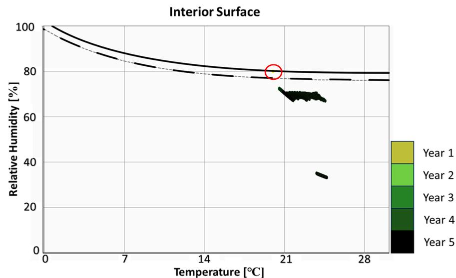
Figure 8. Isopleth graph at different intersection elements in the SW side of the AHW—interior surface.
