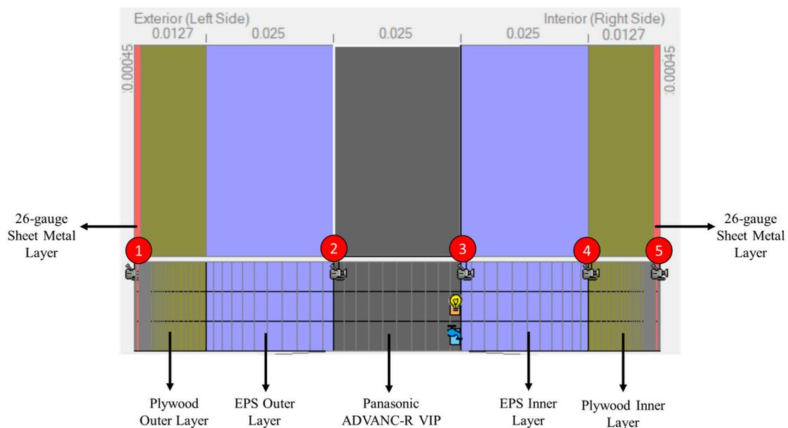
**Figure 4.** Monitoring positions for temperature and RH% using various locations and materials in the adaptable house walls, simulated by WUFI<sup>®</sup>.
