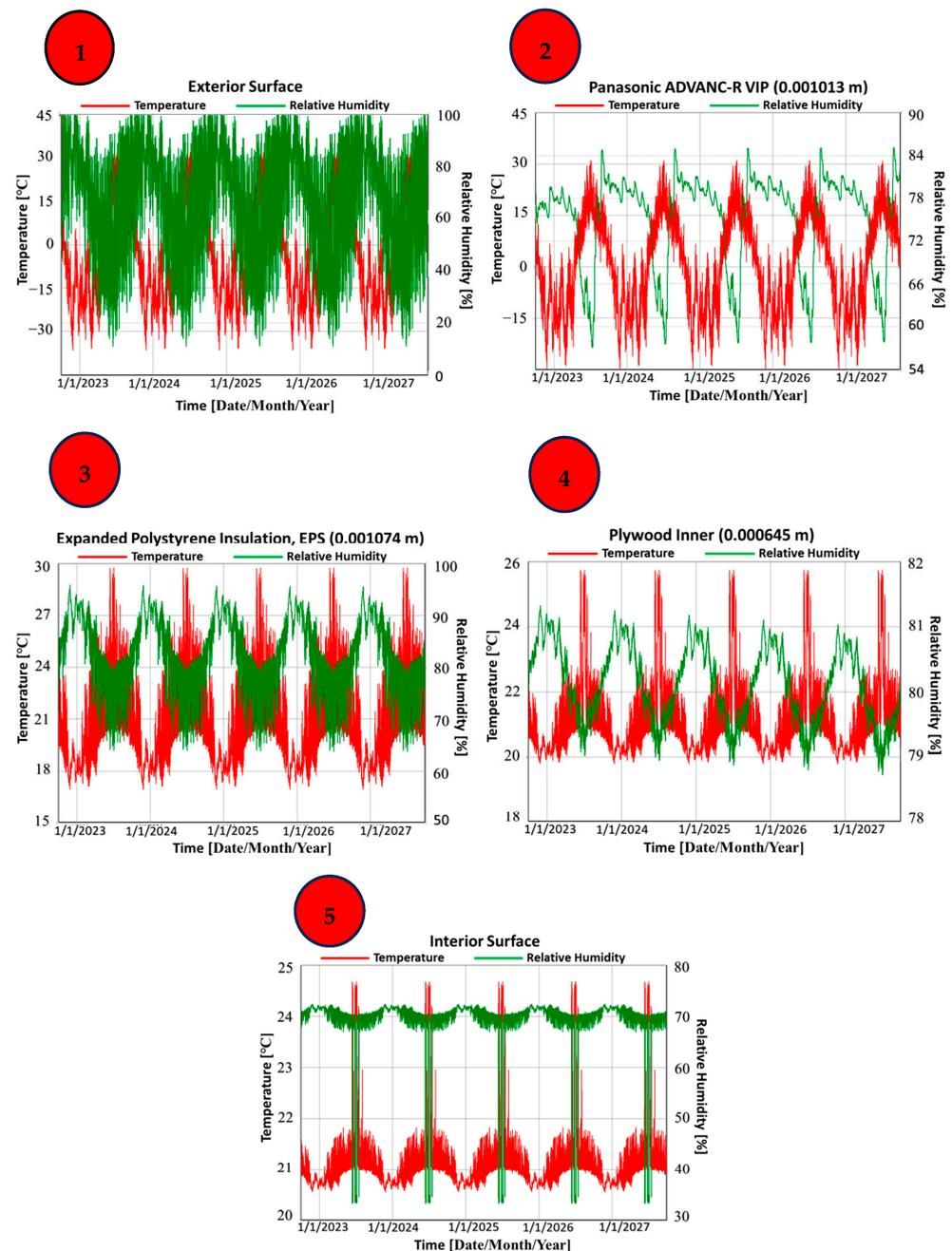
Figure 7. Monitoring temperature and RH% in intersection points between SW wall layers.
