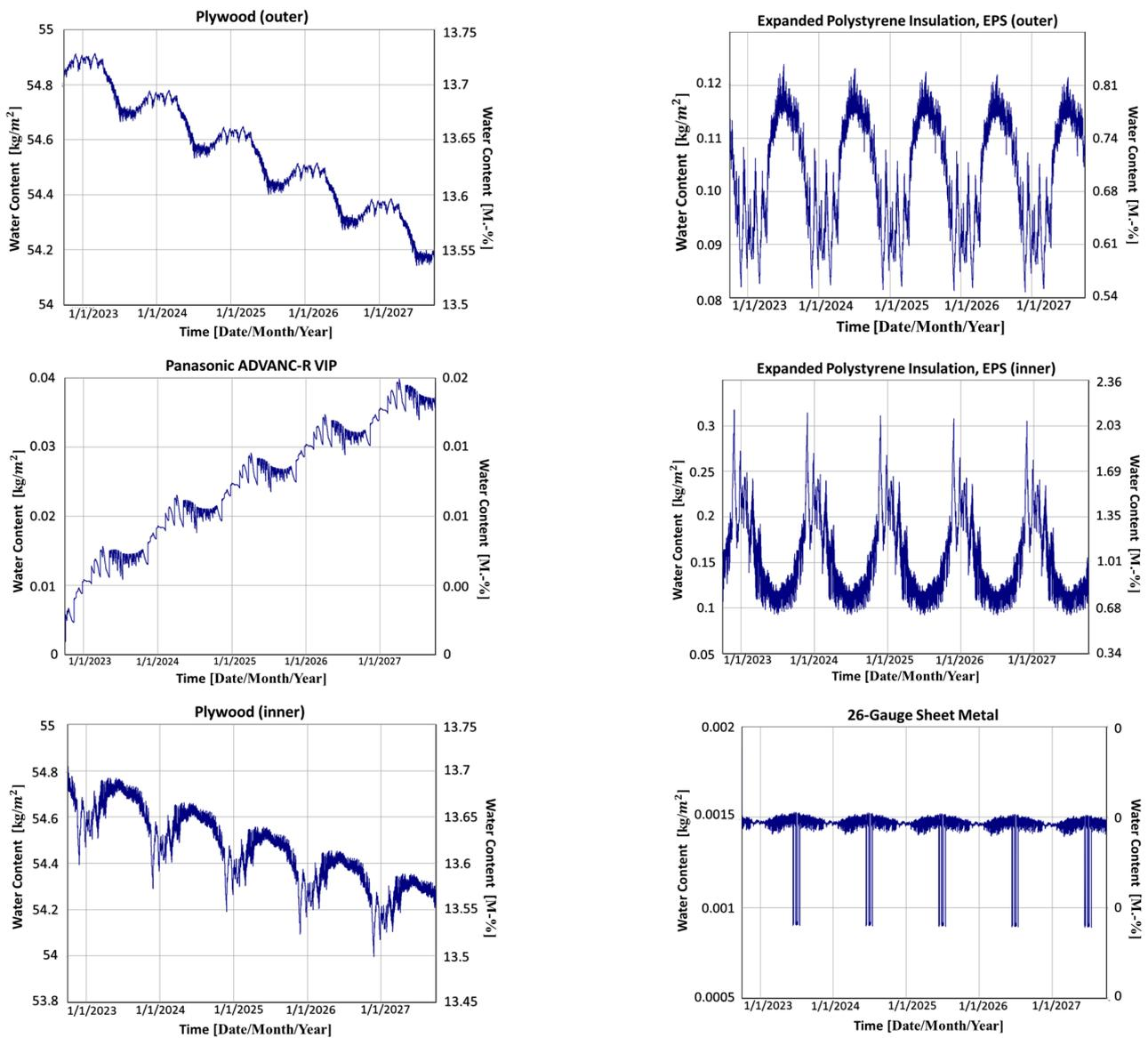
Figure 6. Water content of each material used in the adaptable house SW side wall over the five-year simulation period.
