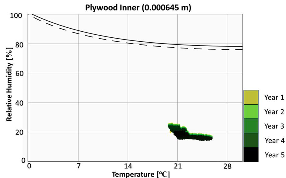
Figure 9. Isopleth graph at different intersection elements in the SW side of the AHW—plywood inner.
