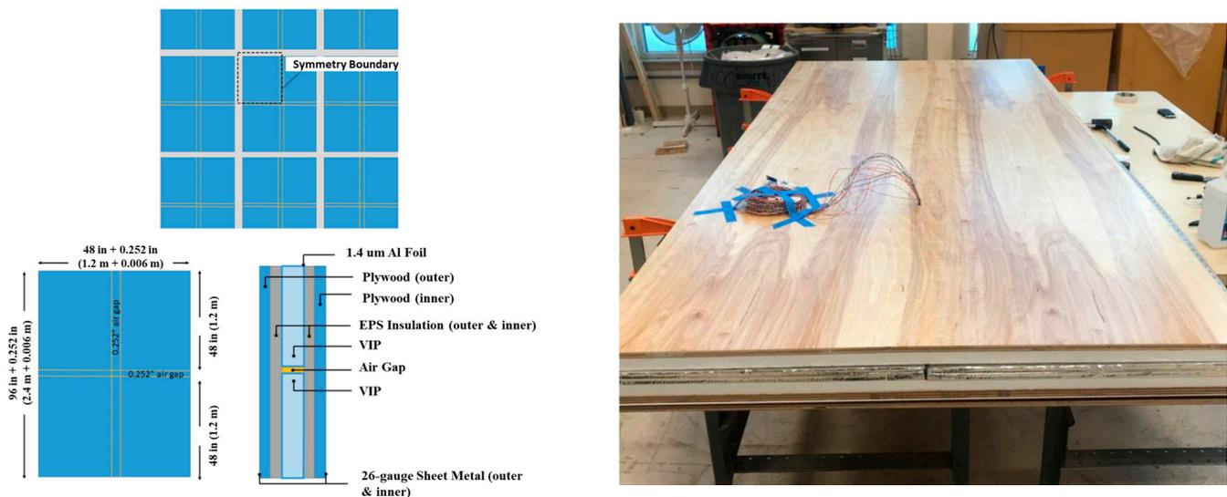
**Figure 2.** Schematic and actual adaptable house wall layout [26].
