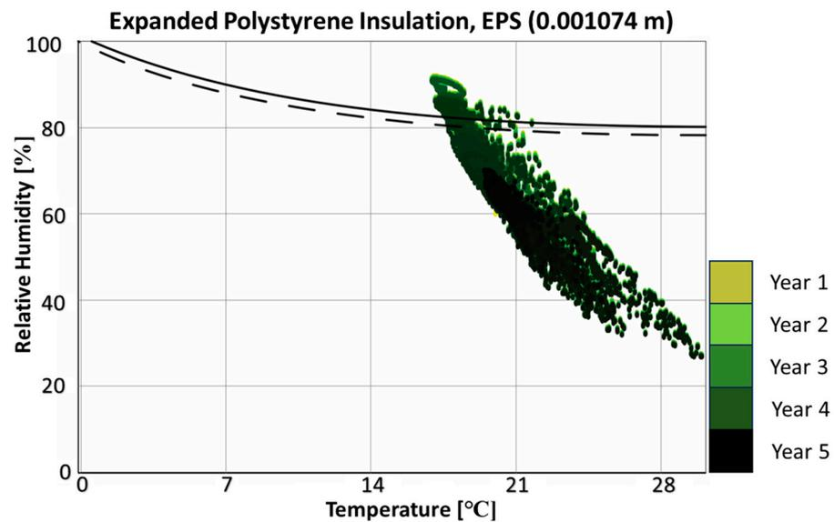
**Figure 10.** Isopleth graph at different intersection elements in the SW side of the AHW—expanded polystyrene insulation (EPS).
