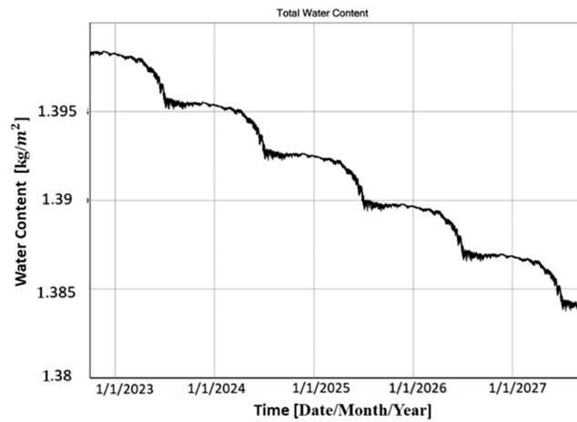
Figure 5. Accumulated moisture content in the SW wall of the adaptable house over a five-year simulation period.
