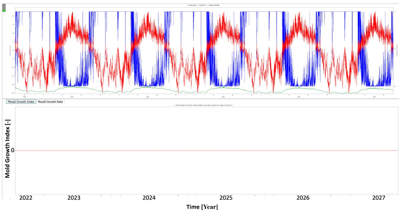
**Figure 14.** Mold growth index (MGI) for the outer plywood layer of the AHWs generated by WUFI® VTT—SW side.
