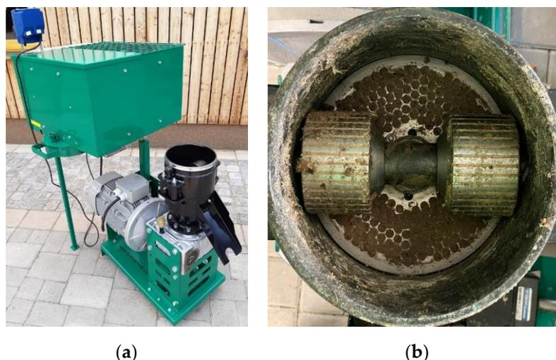
**Figure 3.** (a) BONSAI 100 pelletizer; (b) extrusion rollers and die plate with holes.
