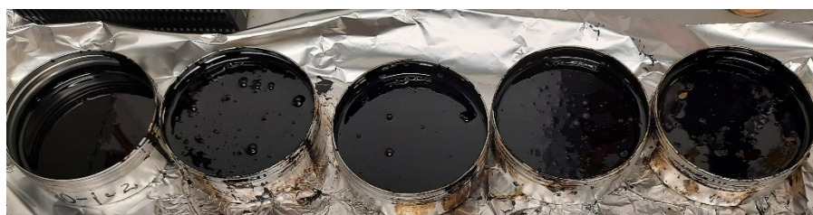
Figure 1. Typical samples of epoxy-modified bitumen.
