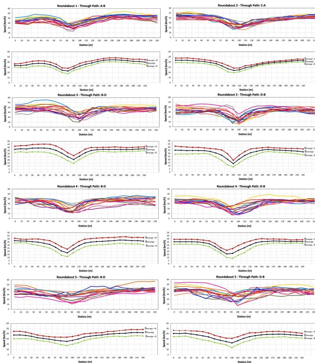
Figure 7. Speed profiles obtained by experimental investigation and representative curves of average speed values and corresponding standard deviations.
