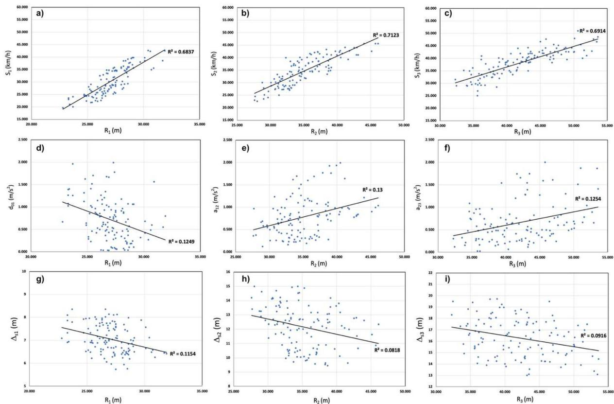
**Figure 8.** Scatter plot of the speed model  $M^{\text{Roundabout}}$  parameters. From subfigure (a–i), blue symbols are the scattered parameter values after model fitting. Black lines are the results after linear regression.
