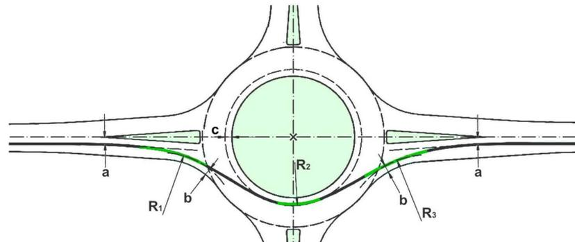
**Figure 2.** Construction of the fastest through path according to the NCHRP model. In this example:  $a = 1.0$  m,  $b = 1.5$  m,  $c = 1.5$  m.
