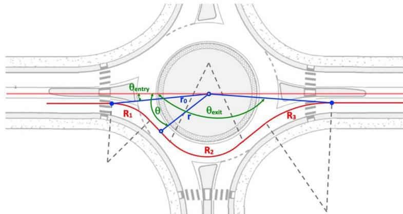
**Figure 3.** Parametric representation of the fastest through path.
