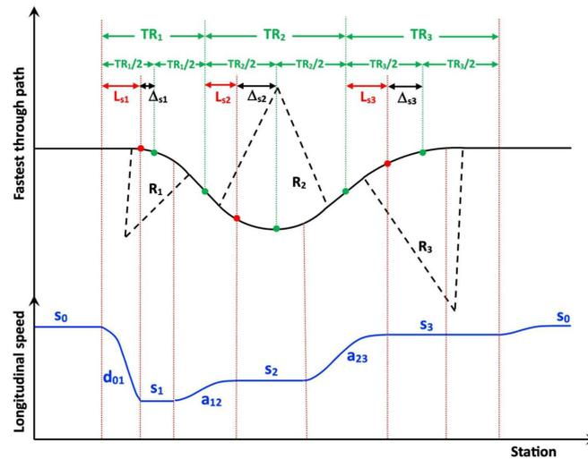
**Figure 4.** Speed model ( $M^{\text{Roundabout}}$ ) to describe the speed profile during the crossing maneuver of a single-lane roundabout.
