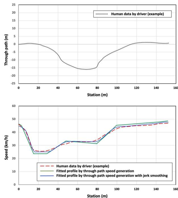
Figure 5. Example of fitting a speed profile by the proposed model ( $M^{\text{Roundabout}}$ ).
