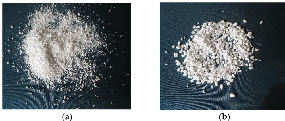
**Figure 1.** Sample pictures: (a) sample PLLA<sub>B2BP</sub> for ecotoxicity test, (b) sample PLLA<sub>B2B3</sub> for disintegration test.
