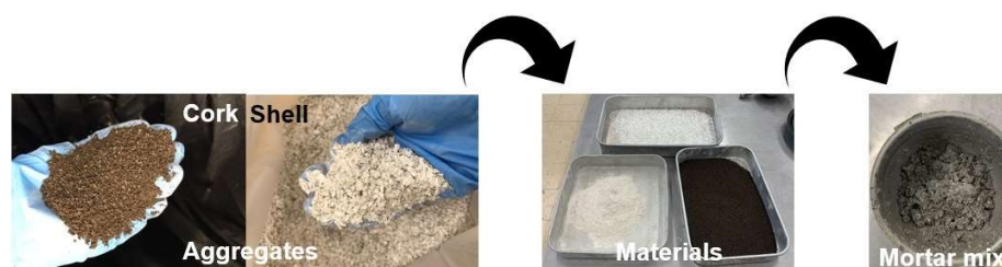
Figure 2. Materials and mortar mix.
