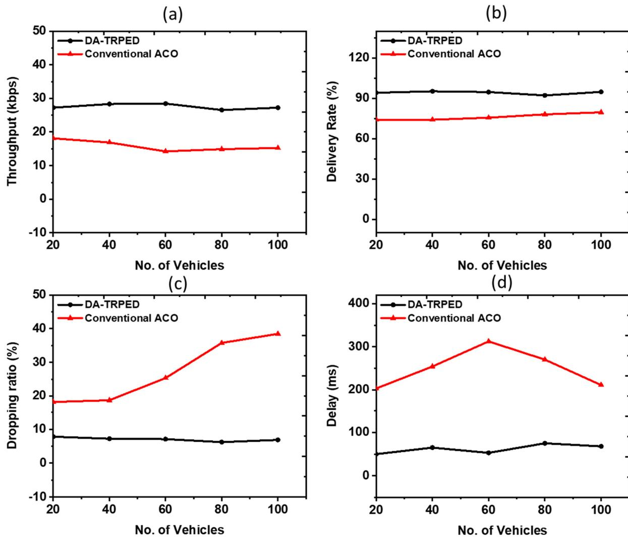
**Figure 4.** Comparative analysis of the existing ACO and proposed DA-TRPED models. (a) Throughput results analysis; (b) packet delivery ratio analysis; (c) packet dropping ratio analysis; (d) end-to-end analysis.
