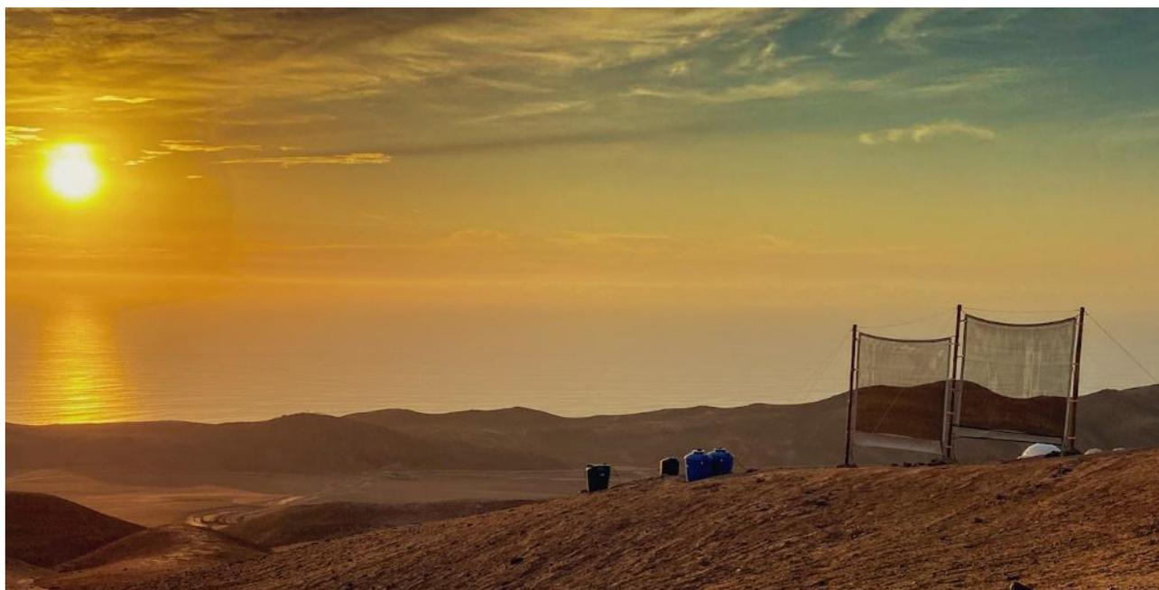
**Figure 1.** Large fog collector installed at the Atacama UC Experimental Station, Alto Patache, coastal Atacama Desert.
