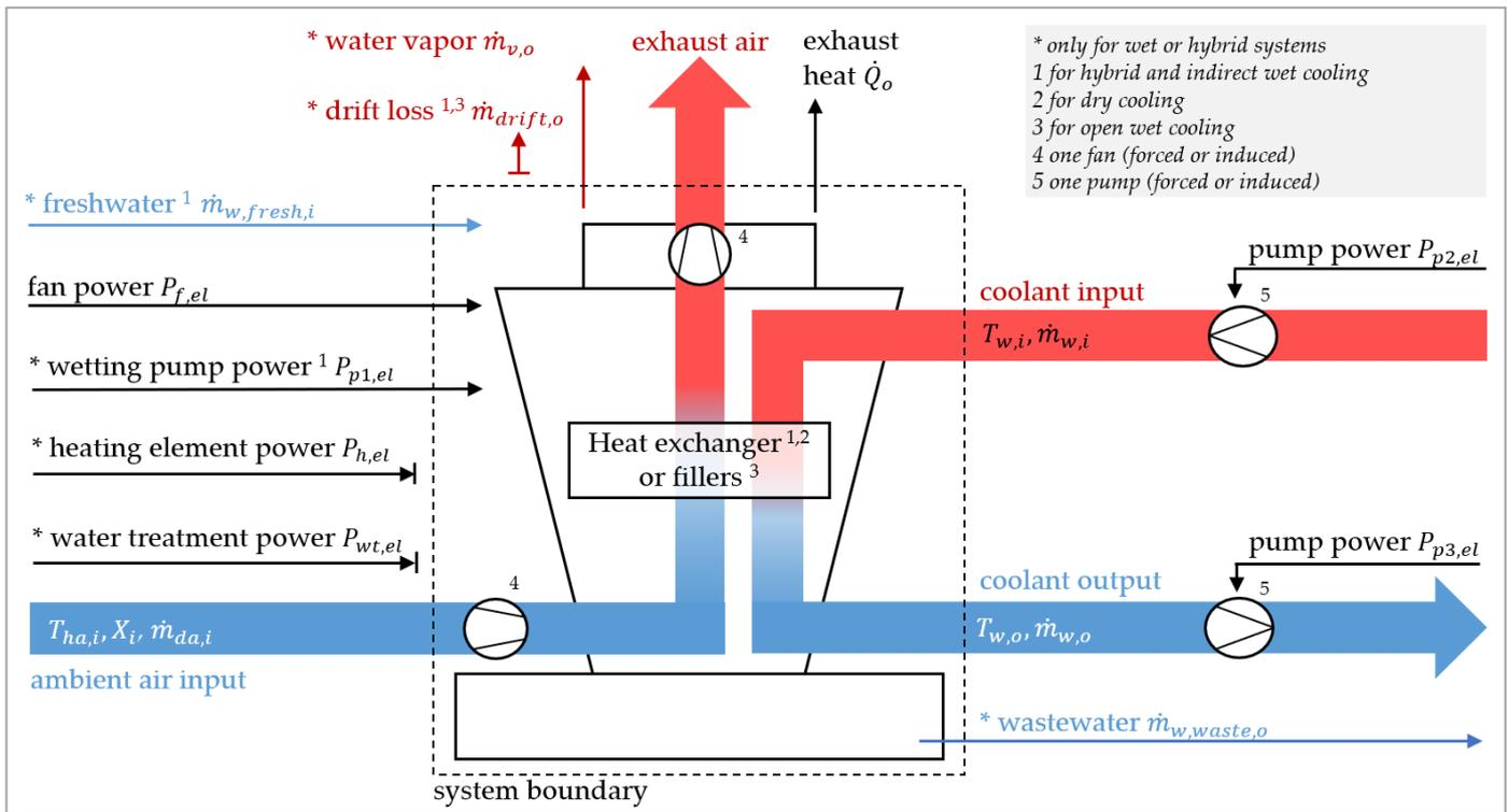
Figure 3. Generalized system boundary of different cooling tower types, based on Wenzel et al. [39]. The cooling tower transfers heat from the coolant flow to the ambient airflow.
