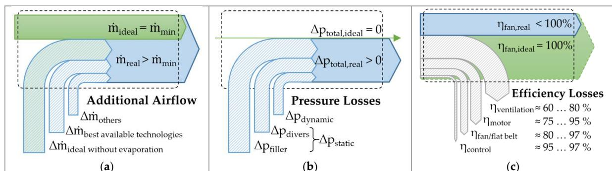
**Figure 11.** Sources of inefficiency in (a) additional airflow, (b) the pressure drop, and (c) the fan efficiency. All three have one physically ideal case (highlighted in green). In practice, technical imperfections cause additional effort or losses (in gray), resulting in the actual situation (in blue). The efficiency values of the ventilation, motor, fan, or flat belt and control system are approximate benchmarks by literature [47,48] (pp. 35–42), [49] (pp. 56–57), [50].
