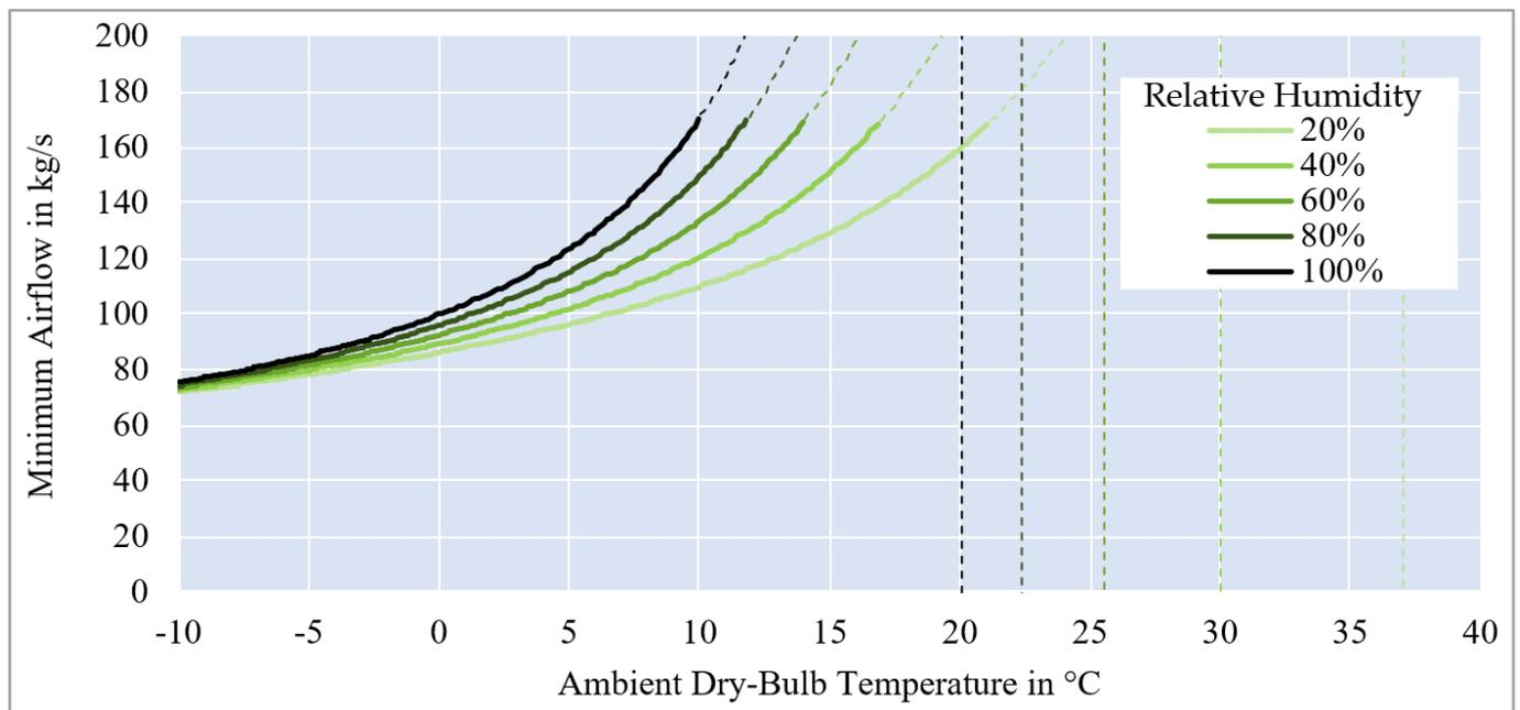
**Figure 5.** Theoretical *minimum airflow* for 4.8 MW<sub>th</sub> heat removal from 20 °C to 10 °C required coolant temperature depending on the outside temperature and humidity. Table S2 in the Supporting Material provides the underlying data.
