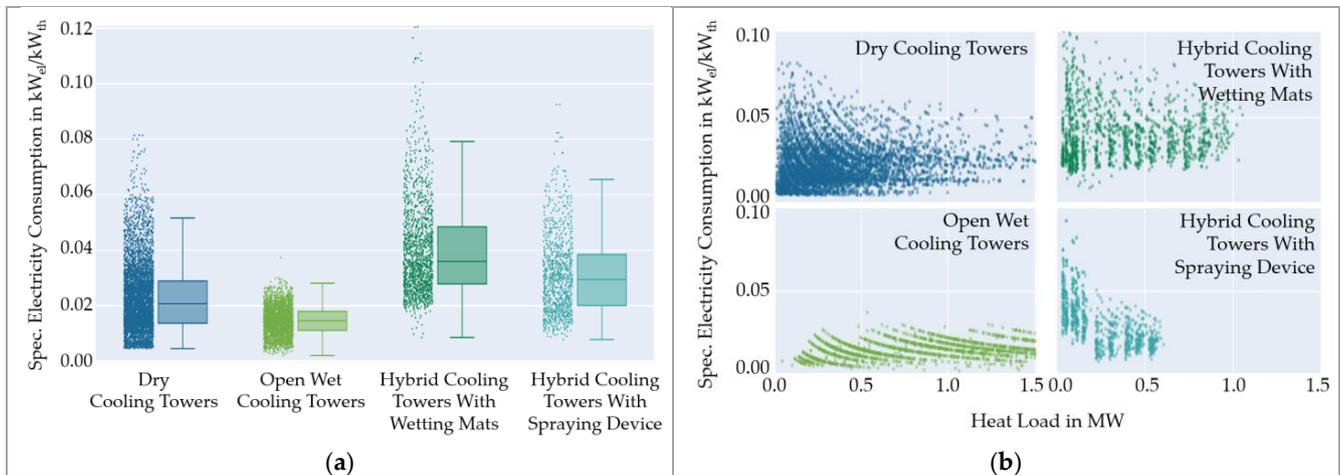
**Figure 8.** Results for the specific electricity consumption by Wenzel et al. [39] (a) as a boxplot diagram and (b) over the heat load.
