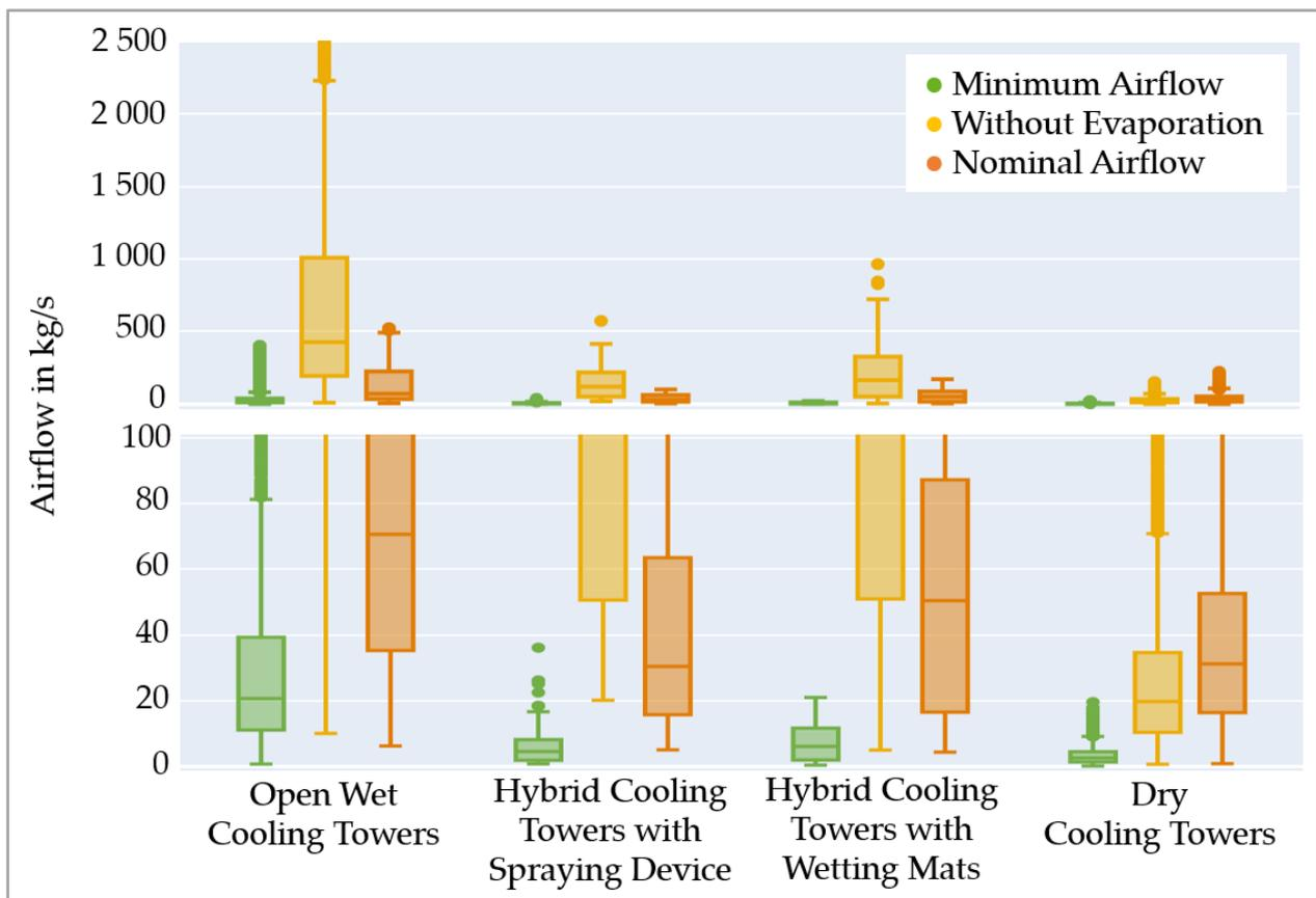
**Figure 6.** *Minimum airflow* (green) compared to the theoretical minimum airflow without evaporation (yellow) and the nominal airflow (orange) of each operating point in the cooling tower dataset. Each type's data consist of 1035 to 5475 operating points (cf. Figure 4). Table S3 in the Supporting Material provides the underlying data.
