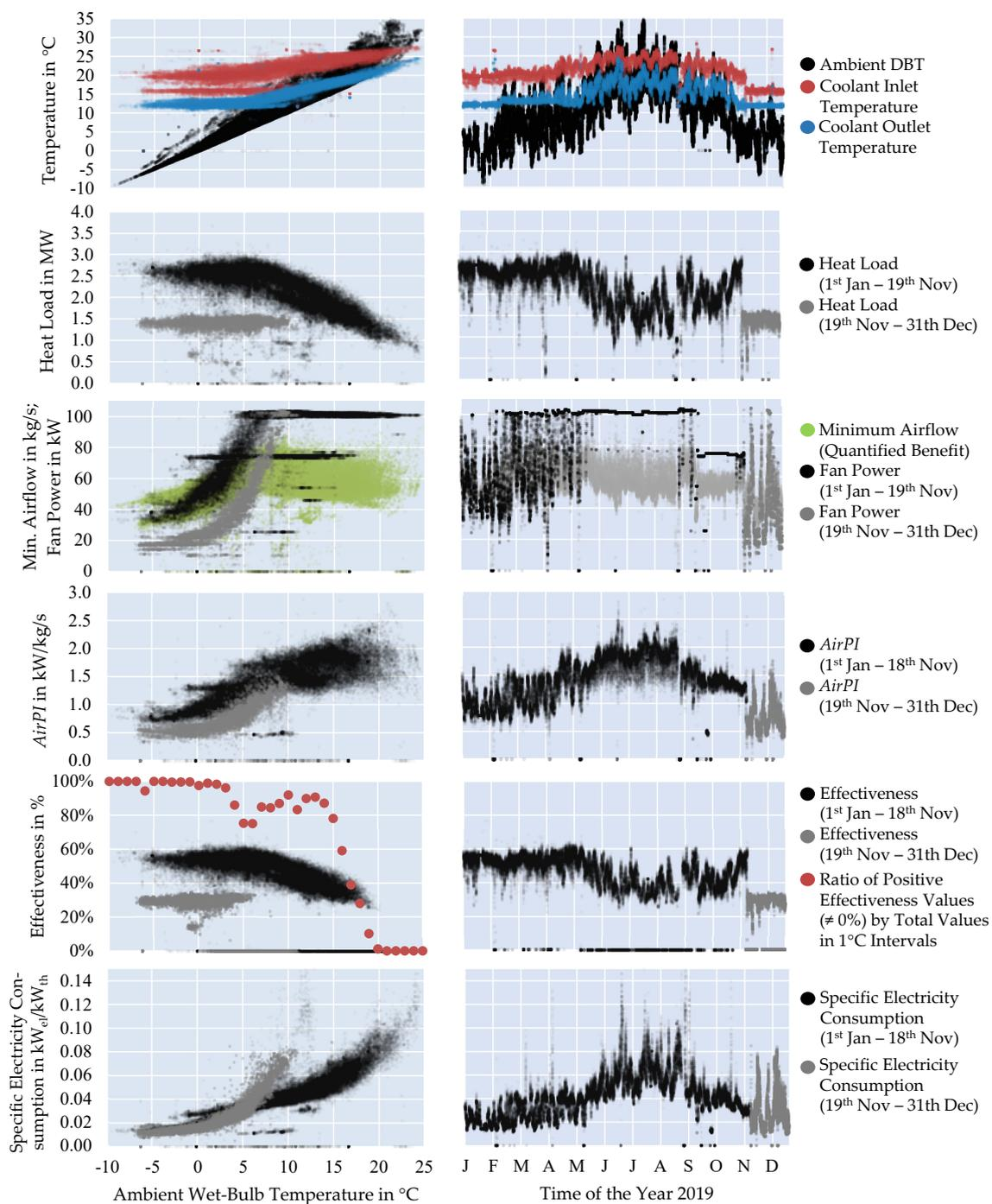
**Figure 10.** Parameters of the HLRS wet cooling system over the ambient WBT and over time: coolant temperatures, ambient DBT, heat load, *minimum airflow*, fan power, *AirPI*, effectiveness referring to the *minimum airflow*, and the specific electricity consumption. Table S5 in the Supporting Material provides the underlying data.
