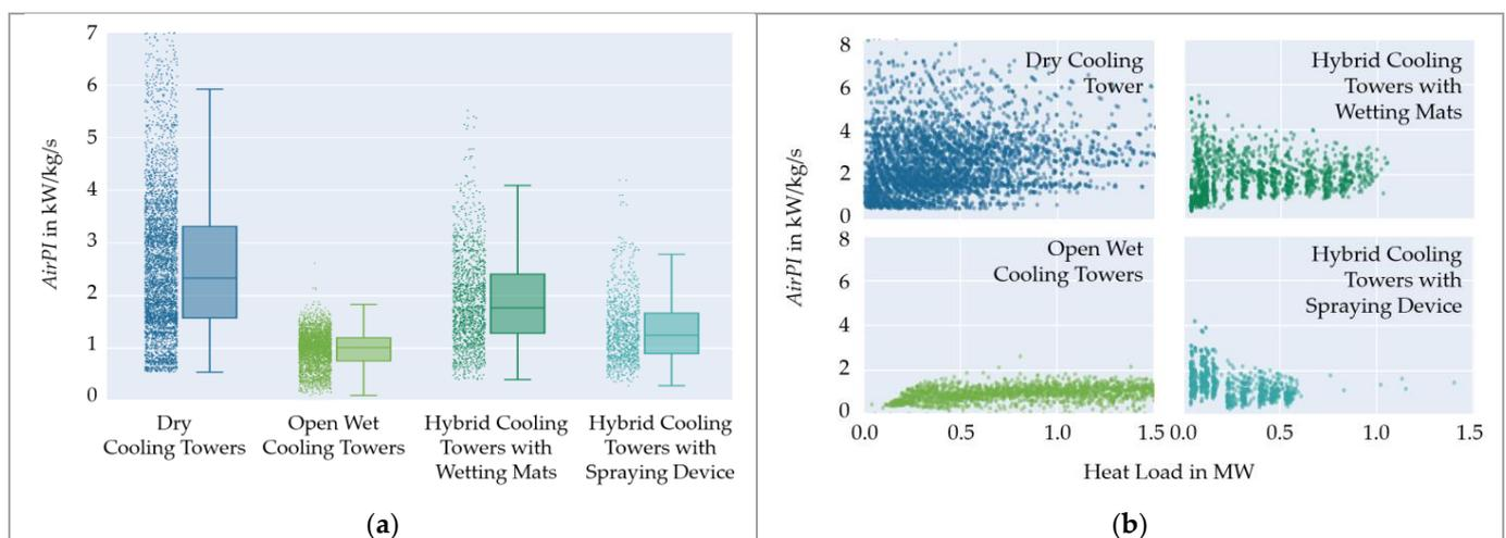
**Figure 7.** *AirPI* results for each cooling tower type (a) as boxplot diagram and (b) over the thermal capacity below  $1.5 \text{ MW}_{\text{th}}$ . Each type's data consist of 1035 to 5475 operating points (cf. Figure 4). Table S4 in the Supporting Material provides the underlying data.
