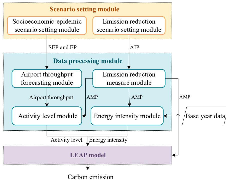
**Figure 2.** LEAP-Airport model framework.
