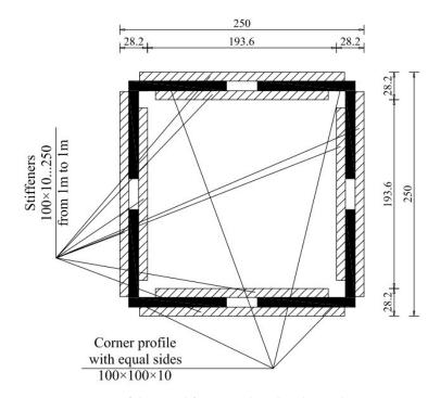
**Figure 4.** Section of the metal frame analyzed in the study— $250 \times 250$  mm.
