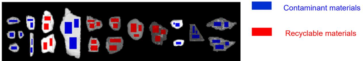
**Figure 3.** Example of different regions of interest (ROIs) selection for class for the two-classes model (i.e., recyclable and contaminants recognition).
