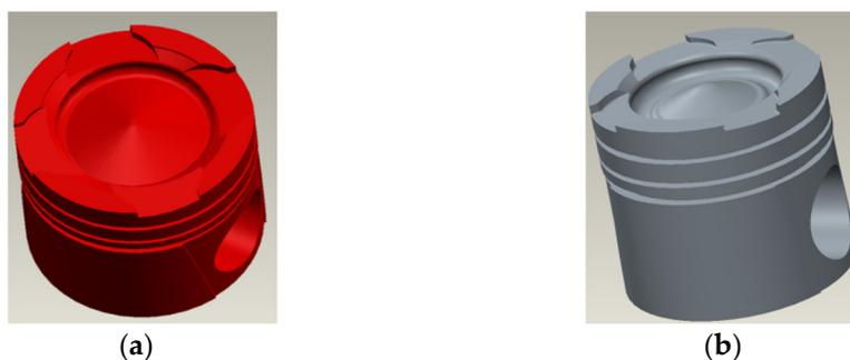
Figure 9. Structures of piston bodies. (a) Baseline. (b) LGFC.
