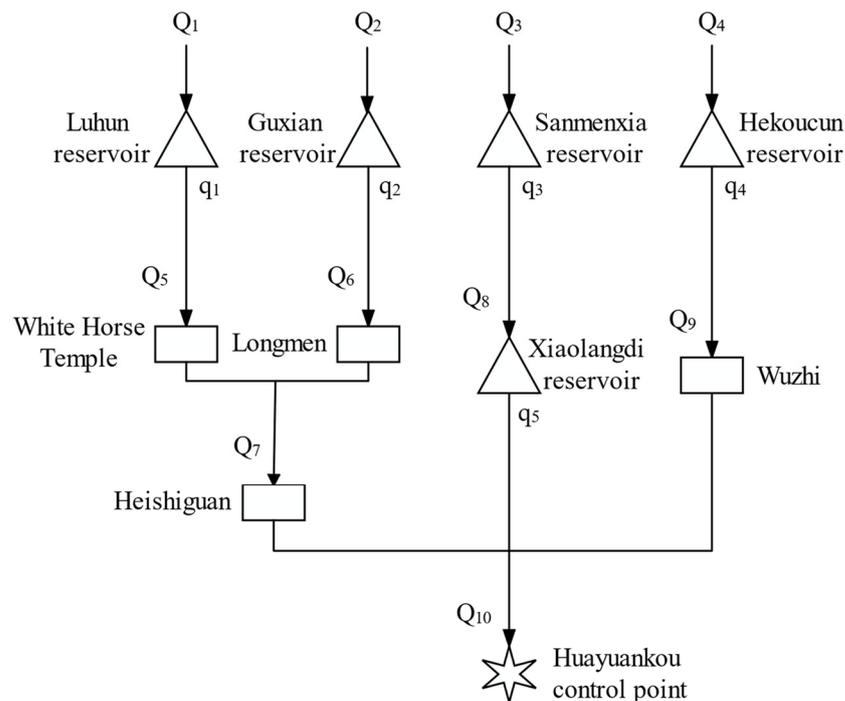
**Figure 1.** Schematic diagram of flood composition of the Huayuankou section.
