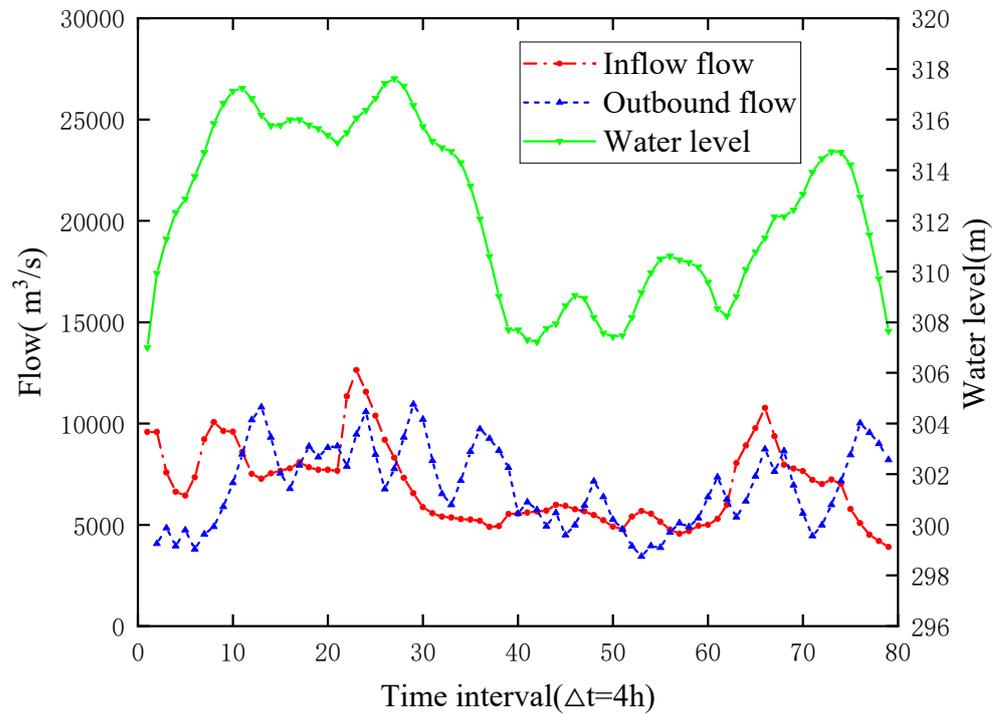
Figure 6. Operation process of Sanmenxia reservoir.
