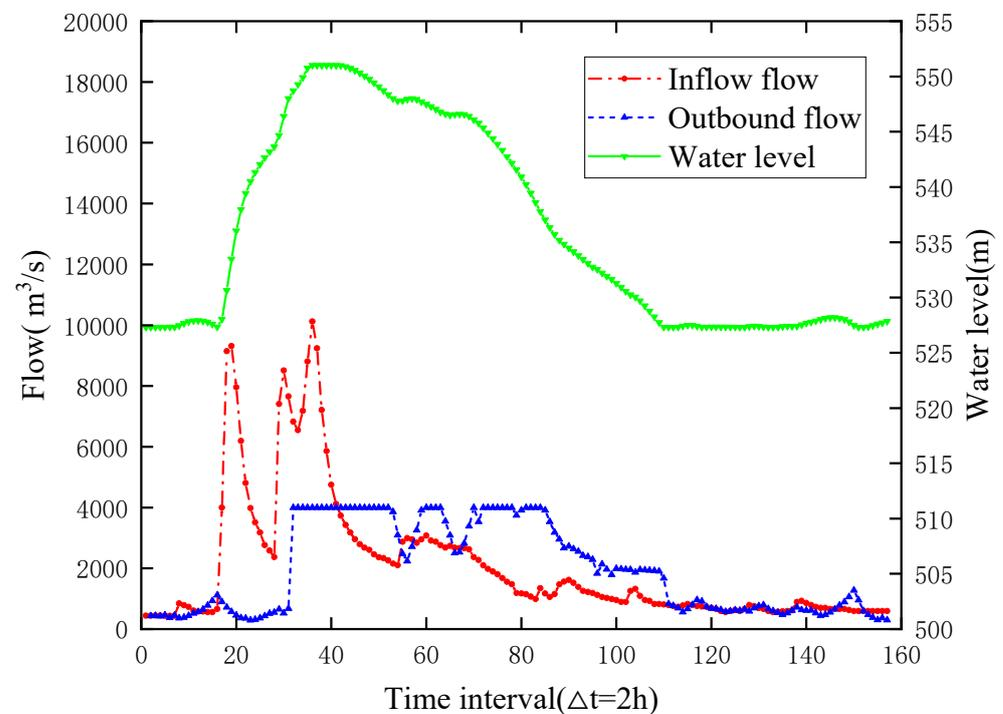
Figure 4. Operation process of Guxian reservoir.
