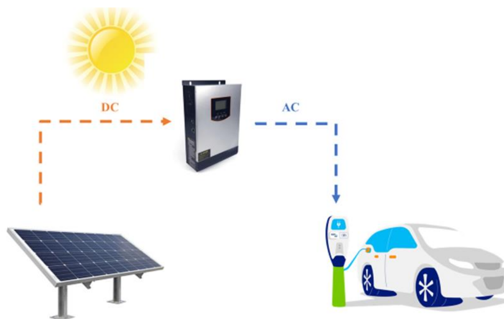
Figure 14. Schematic of a solar charger for EVs.
