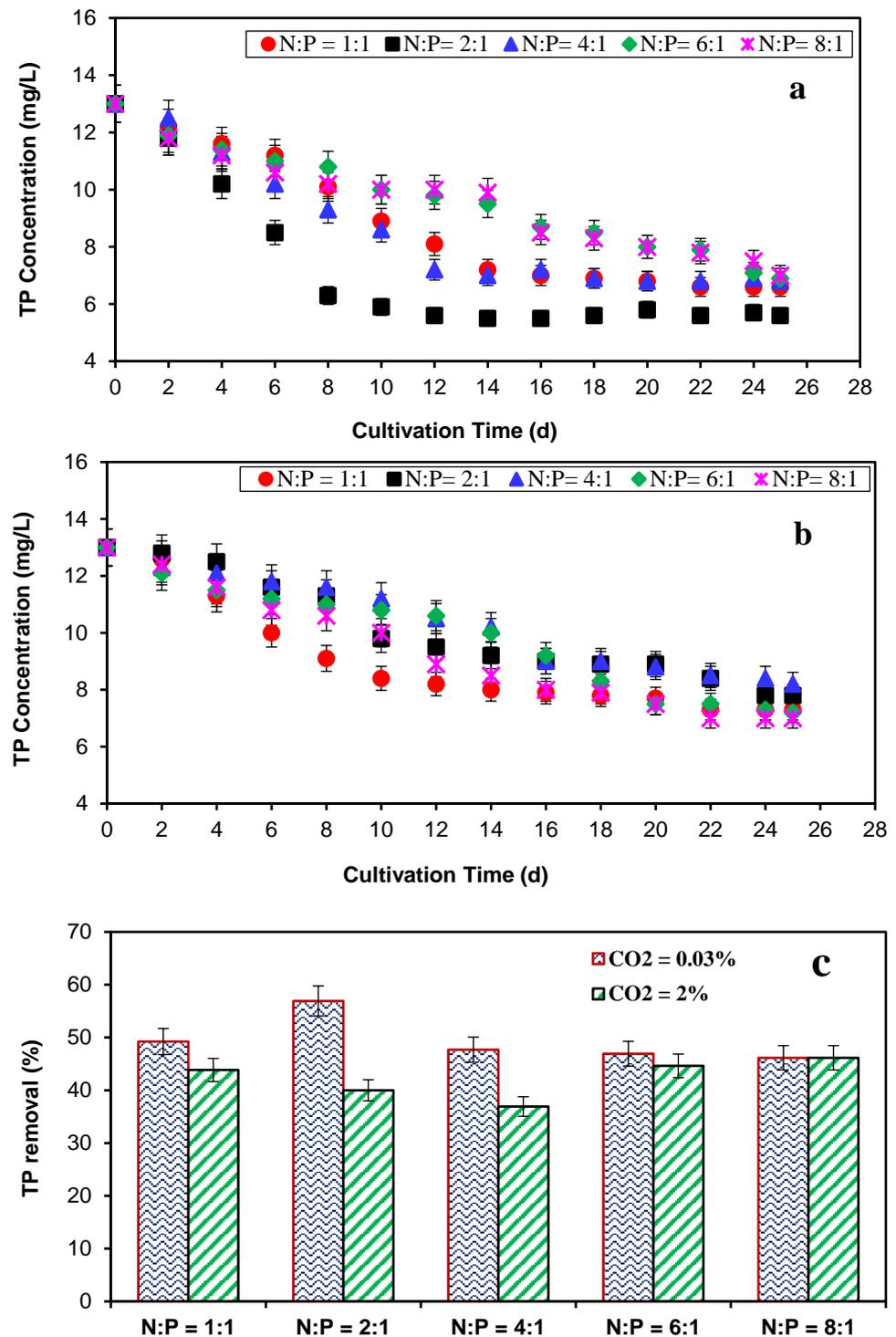
**Figure 6.** Time profiles of the effect of the total phosphorous (TP) concentration on *Scenedesmus dimorphus* cultivated under different levels of nitrogen-to-phosphorous (N:P) ratios (a) without CO<sub>2</sub> supplementation (air only) and (b) with CO<sub>2</sub> supplementation (2% CO<sub>2</sub> in air). (c) A comparison of the removal of total phosphorous (TP) under the experimental conditions of this study. Data are means  $\pm$  SD ( $n = 3$ ).
