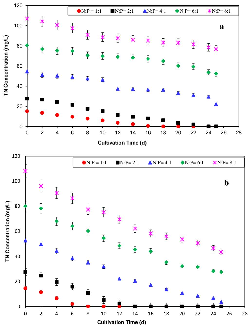
**Figure 5.** Time profiles of the effect of the total nitrogen (TN) concentration on *Scenedesmus dimorphus* cultivated under different levels of nitrogen-to-phosphorous (N:P) ratios (a) without CO<sub>2</sub> supplementation (air) and (b) with CO<sub>2</sub> supplementation (2% CO<sub>2</sub> in air). Data are means  $\pm$  SD ( $n = 3$ ).
