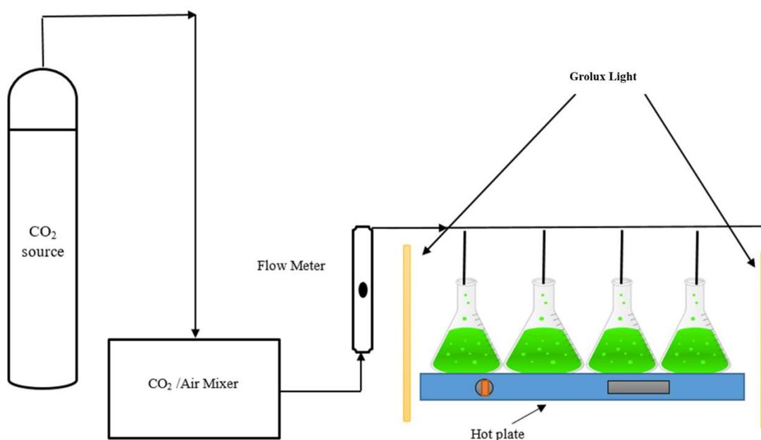
**Figure 1.** A schematic diagram of the experimental set up (adapted from Razzak 2019, accessed on 20 January 2019).
