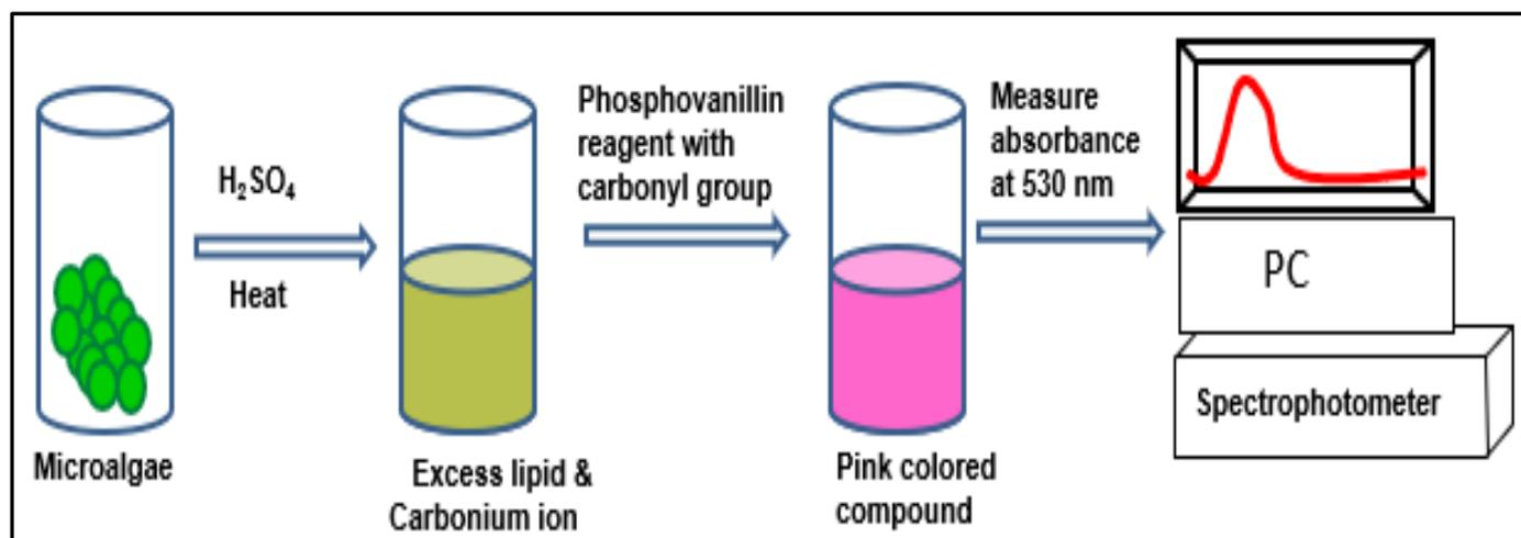
**Figure 2.** A schematic representation of the lipid detection principle in the SPV-based colorimetric assay (adapted from Razzak 2018, accessed on 24 February 2019).
