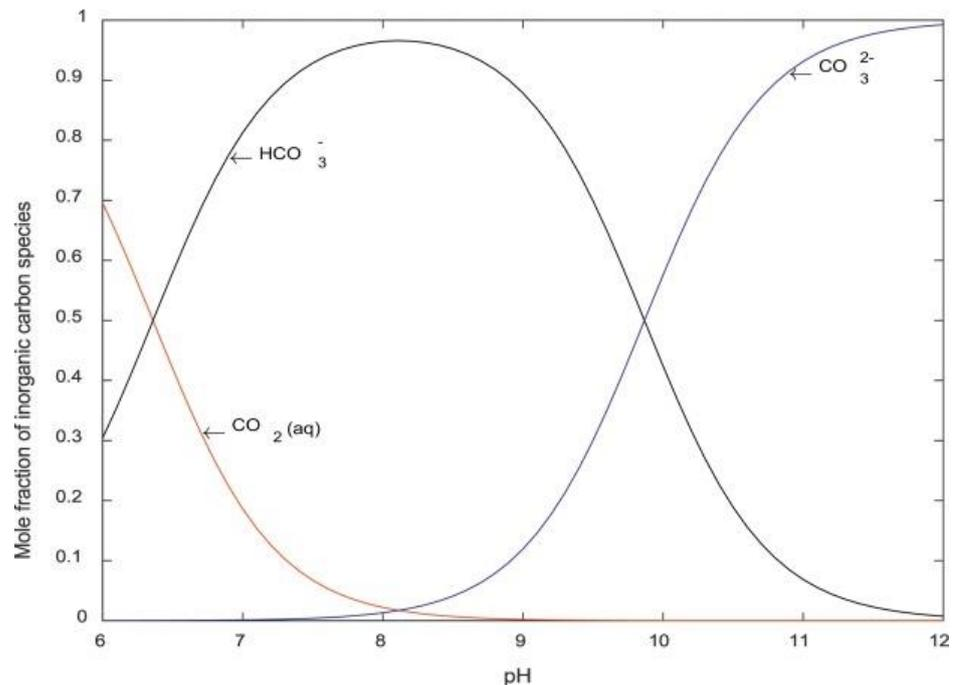
**Figure 7.** Different inorganic carbon species with respect to mole fractions at different media pH (adapted from Eze et al. 2018, accessed on 15 April 2019).
