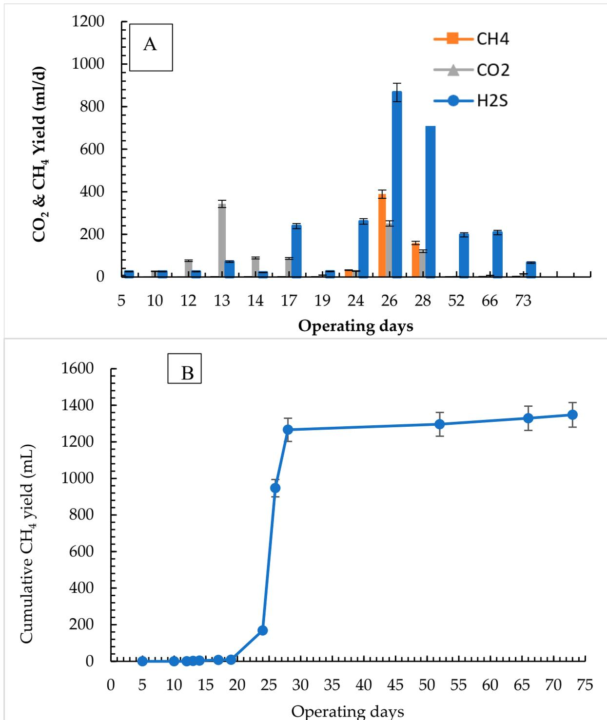
**Figure 6.** Biogas yield in R1 (A). Cumulative methane yield in R1 (B).
