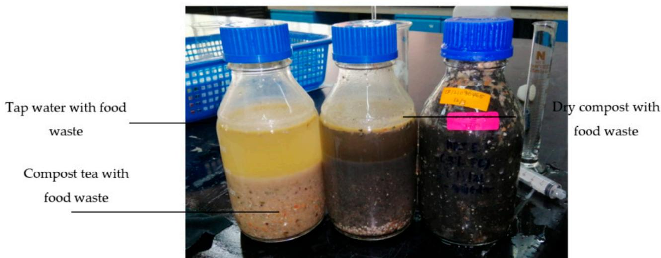
**Figure 1.** Substrate mixture to study compost as a pH buffering biomaterial.
