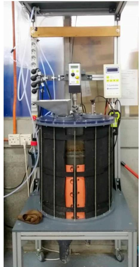
**Figure 2.** Schematic diagram and photo of Umwelteleistungen biogas test plant standard (BTP2). “1” refers to gas bag, “2” refers gas outlet valve, “3” refers to substrate inlet, “4” is meter, “5” is mixer blade, “6” is pH meter, “7” thermometer for substrate, “8” thermometer for gas, “9” large substrate outlet, and “10” small substrate outlet.
