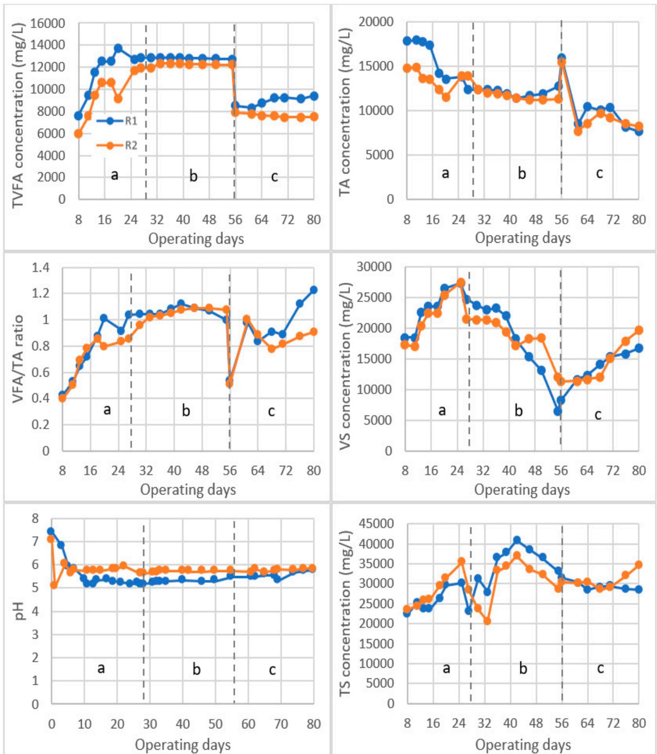
**Figure 7.** Parameter changes of Reactor 1 (R1, blue colour) and Reactor 2 (R2, red colour) across 3 stages. “a” refers to biogas production stage, “b” refers to acidification stage, “c” refers to compost addition stage.
