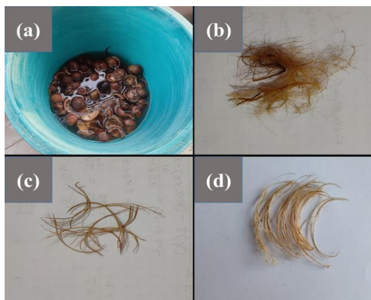
Figure 3. Areca fiber extraction process: (a) soaked areca nut husk, (b) mixed fibers, (c) extracted coarse fibers, (d) saturated surface dry fiber (before mixing).
