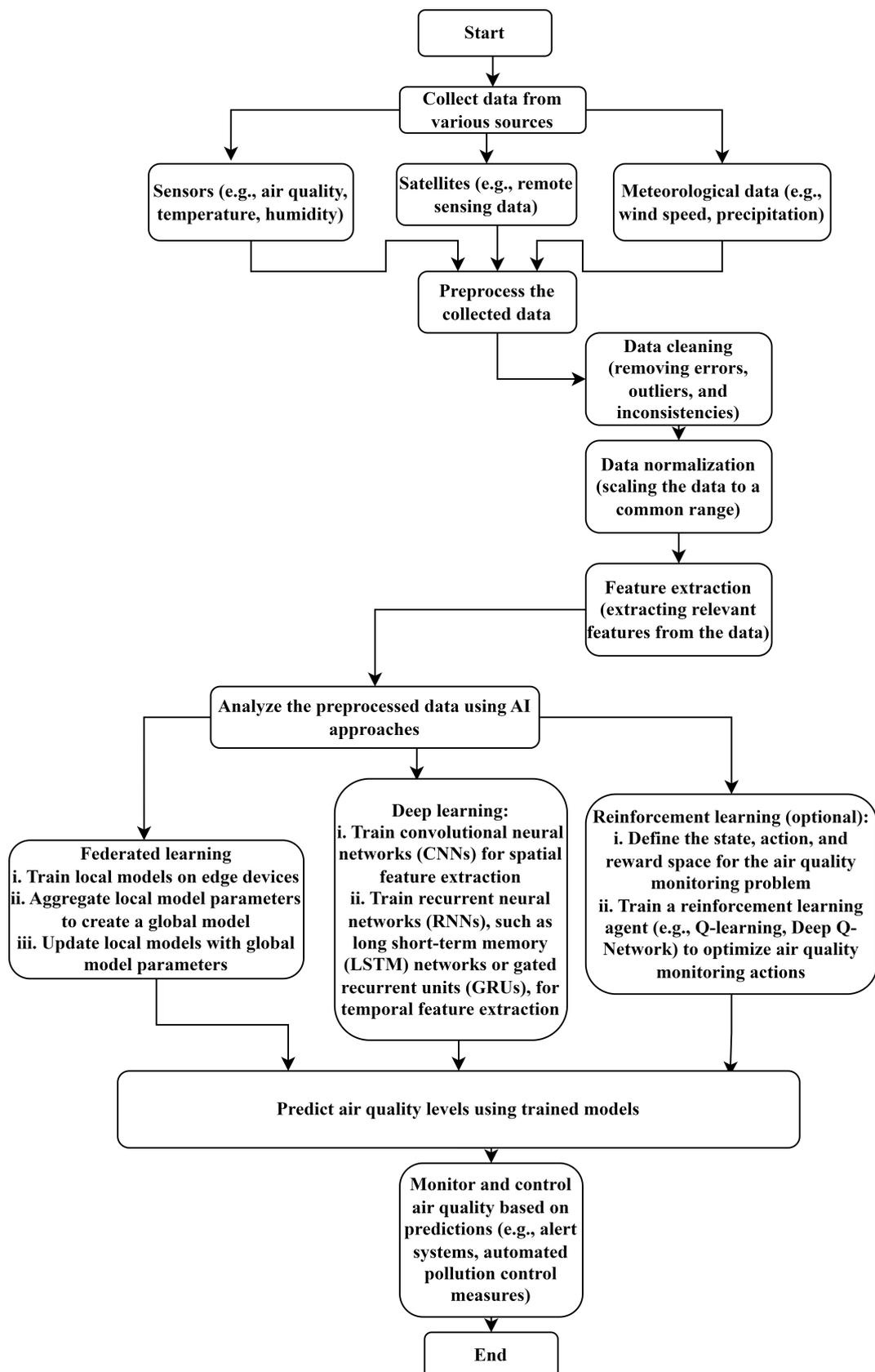
**Figure 5.** Flowchart for collecting, preprocessing, analyzing, and predicting air quality data using edge computing and AI approaches.
