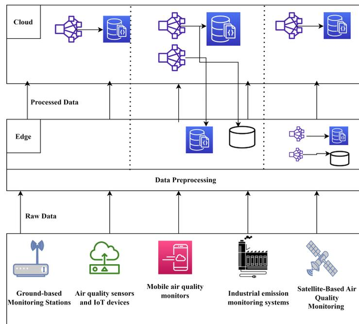
**Figure 4.** Air quality monitoring system supported by Internet of Things for data collection and processing [61].
