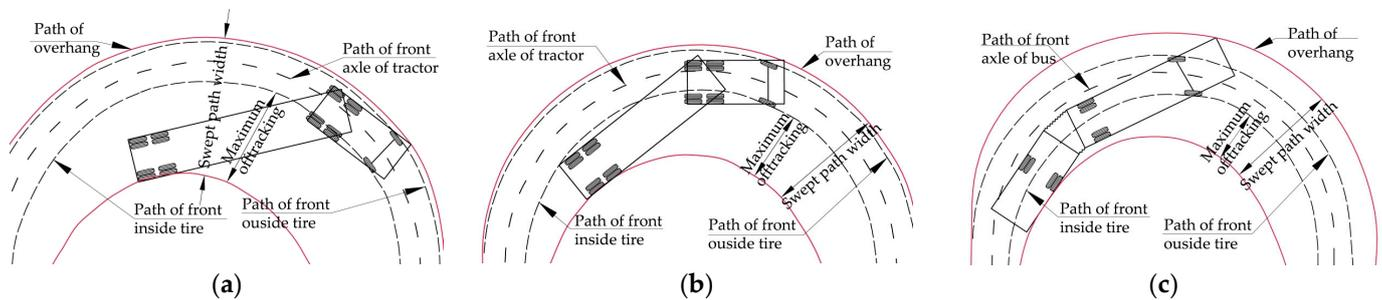
**Figure 4.** Turning characteristics of selected design vehicle: (a) DV1; (b) DV2; (c) DV3. Source: own work.
