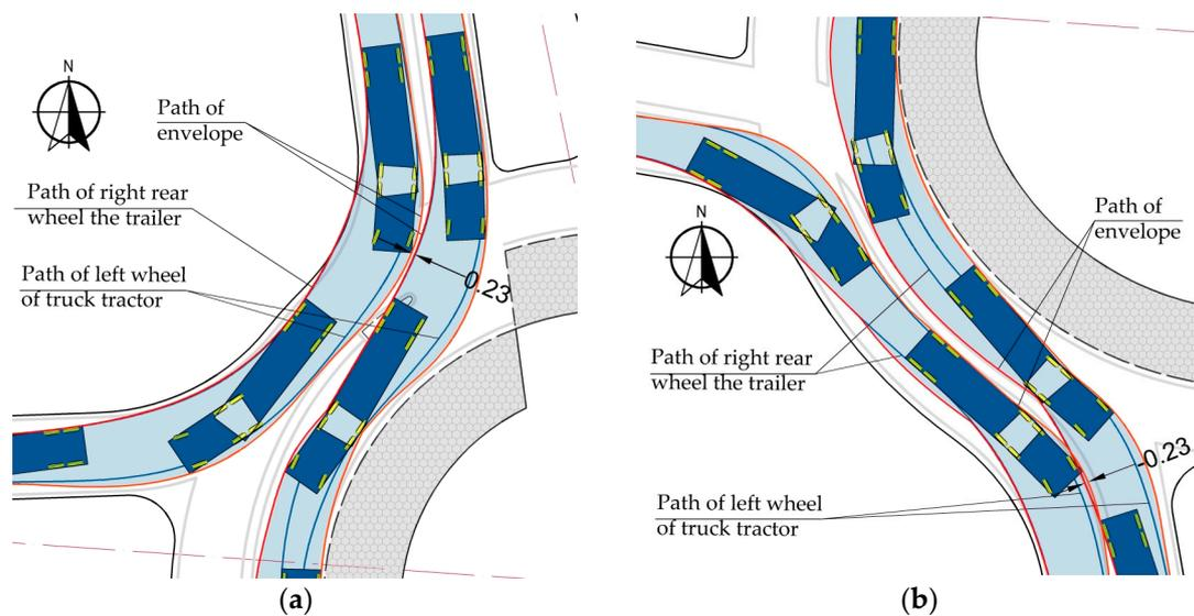
**Figure 7.** Analysis of the swept paths of the shortest design vehicle (DV2): (a) north entry; (b) west entry (units in m). Source: own work.
