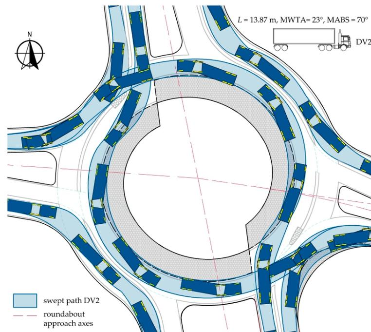
**Figure 8.** Selected swept paths of DV2 following a change in the roundabout geometry that involved primarily widening the circulatory lanes. Source: own work.
