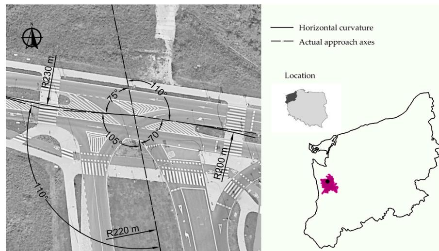
**Figure 1.** The alignment of the approach axes at the location selected for the described analyses of the proposed turbo-roundabout. Source: authors' elaboration against the background of the satellite photograph from z [40].
