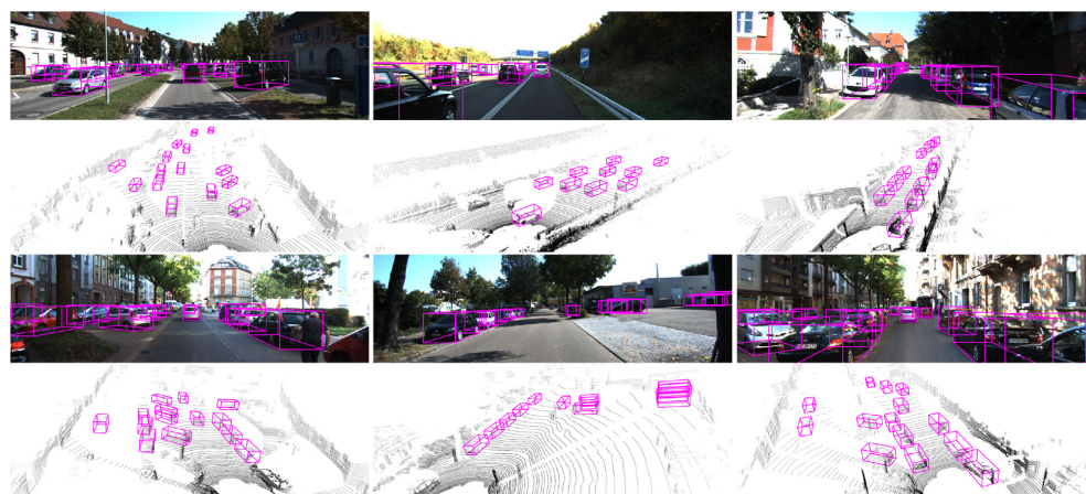
Figure 5. KITTI dataset visualization and prediction results. Sub-figures show predictions for PointPillars and SECOND RPNs at various angles with the DFA-SAT 3D object detection approach.
