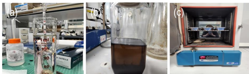
Figure 4. Density separation method using the standard solution: (a) Liquid separation tester, (b) density separation, and (c) sample drying.
