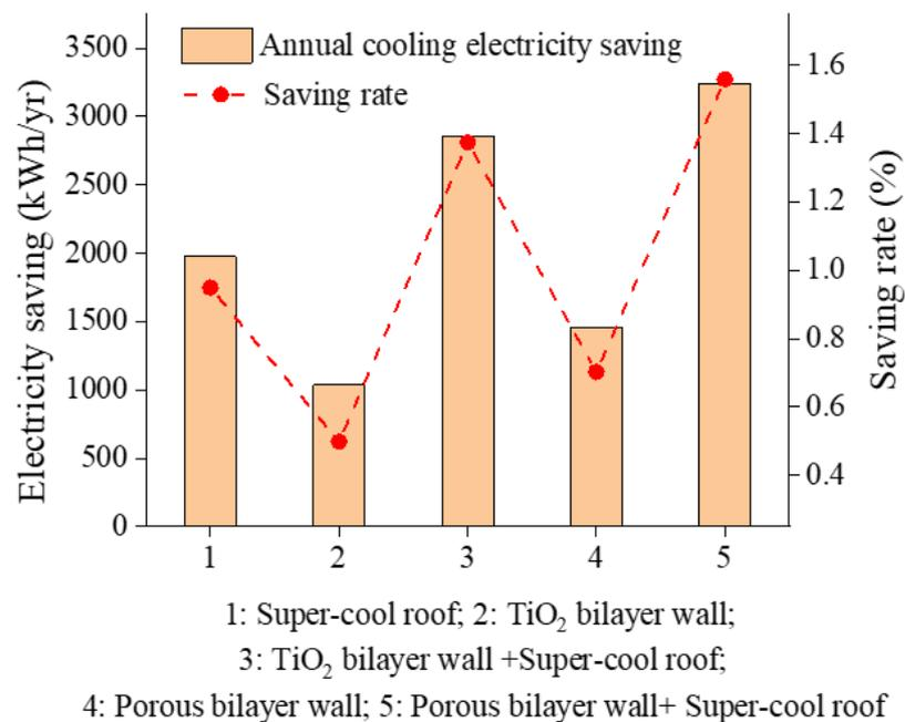
Figure 12. Yearly cooling electricity saving and saving rate relative to the monolayer wall.
