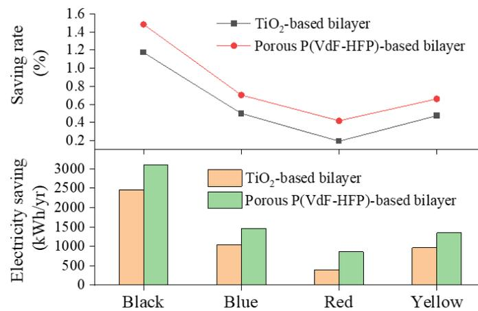
Figure 5. Cooling electricity saving relative to the monolayer wall with the same color.
