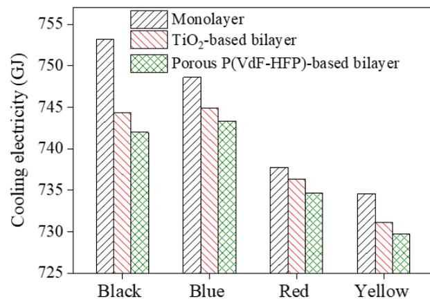
Figure 4. Cooling electricity consumption induced by differently colored cooling walls.
