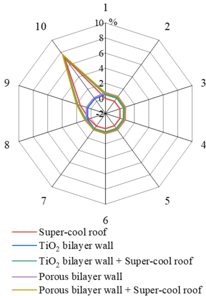
Figure 11. Yearly cooling electricity saving rate in each floor relative to the monolayer wall.
