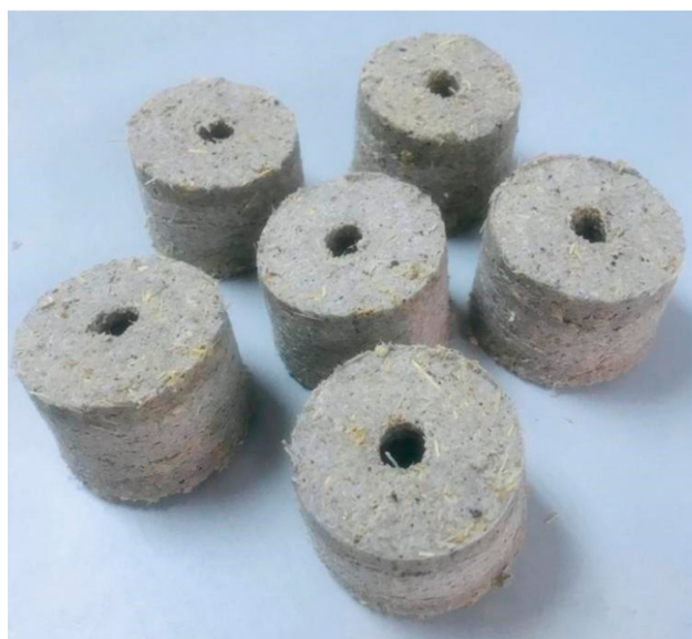
Figure 9. Example of briquettes made with a manual piston press [144].
