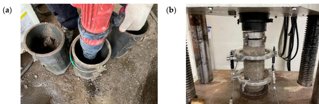
**Figure 8.** Testing method: (a) vibrating hammer test and (b) compressive strength test.
