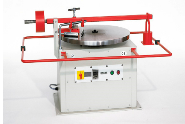
Figure 1. Böhme abrasion test device: 1—counterweight, 2—test track, 3—loading weight, 4—sample holder, 5—tested sample, 6—rotating disc [13,15].
