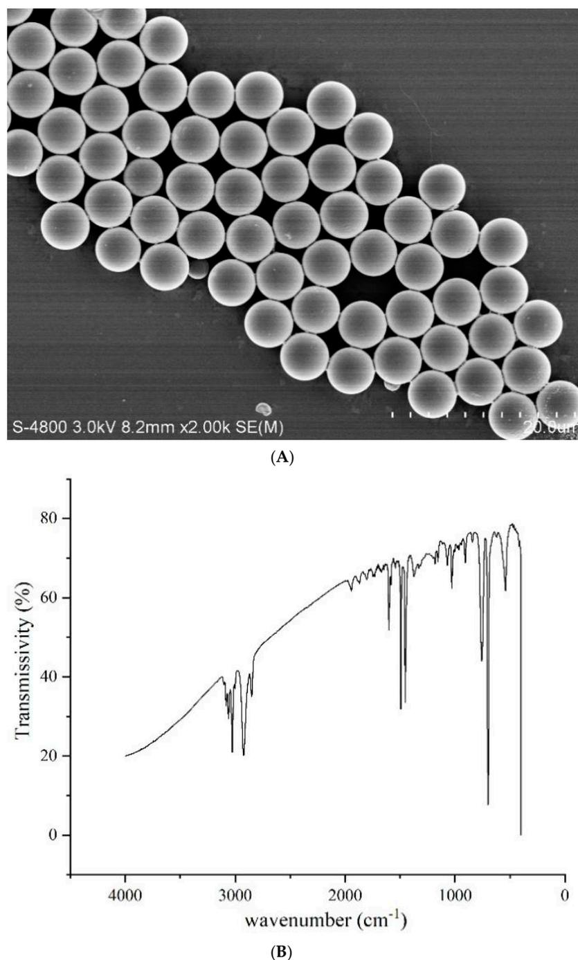
**Figure 1.** The SEM image (A) and FT-IR spectra (B) of PS-MPs.
