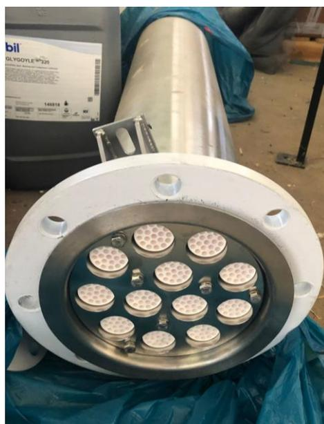
**Figure 1.** Microfiltration unit.
