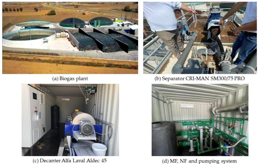
**Figure 2.** Photographs of (a) biogas plant; (b) mechanical separator; (c) centrifugal separator; and (d) microfiltration and nanofiltration units.
