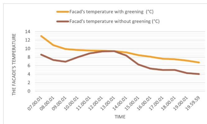
**Figure 6.** Comparing the surface temperature of the southeast façade with and without greening on a winter day.
