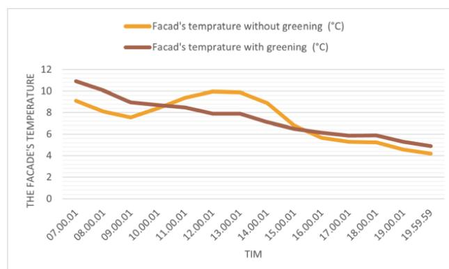
**Figure 8.** Comparing the surface temperature of the northwest façade with and without greening on a cold day.
