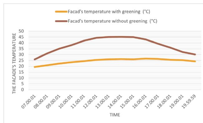
**Figure 7.** Comparing the surface temperature of the northwest façade with and without greening on a summer day.
