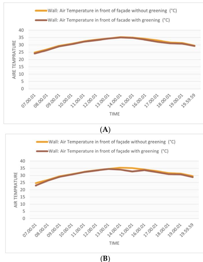
**Figure 13.** (A) Air temperature in front of the southeast façade on a hot day. (B) Air temperature in front of the northwest façade on a hot day.
