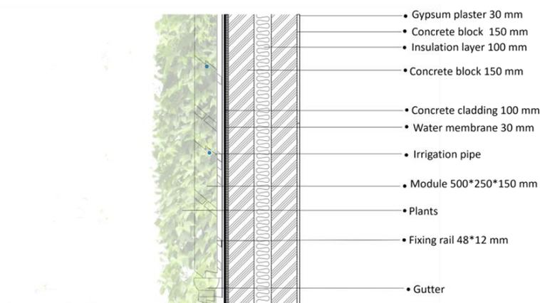
**Figure 3.** Section through the modular living wall system.
