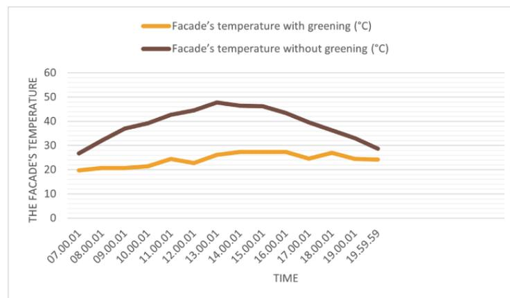
**Figure 5.** Comparing the southeast façade's surface temperature on a summer day in July with and without greening.
