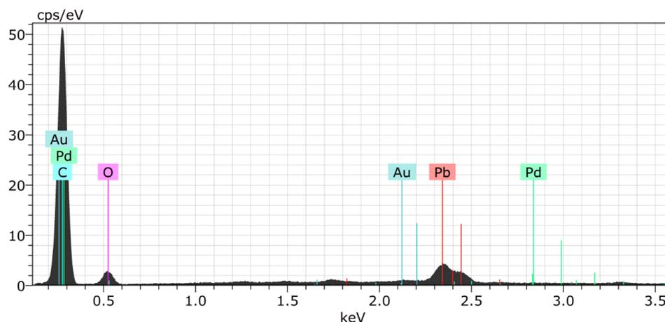
Figure 5. EDX spectra of vine shoot activated carbon.
