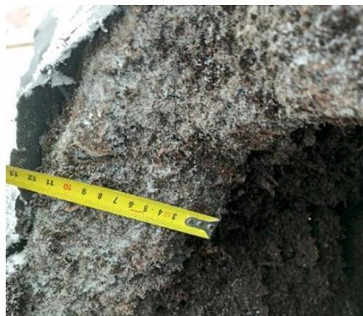
**Figure 4.** The depth of freezing in the heap at atm. air T of  $-14\text{ }^{\circ}\text{C}$ .
