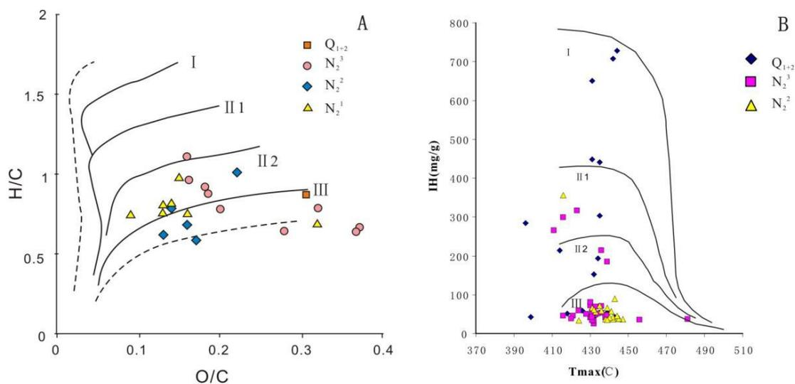
**Figure 4.** Classification of organic matter by elemental analysis. (A) Relation between O/C and H/C of kerogen. (B) Relation between hydrogen index of kerogen and pyrolysis T<sub>max</sub>.
