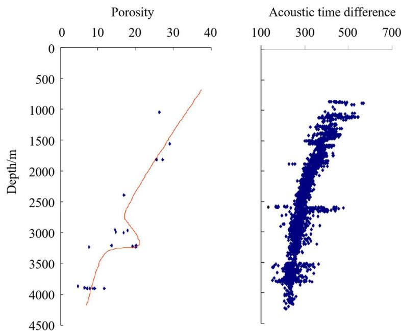
**Figure 7.** The relationship between porosity and acoustic time difference with depth.
