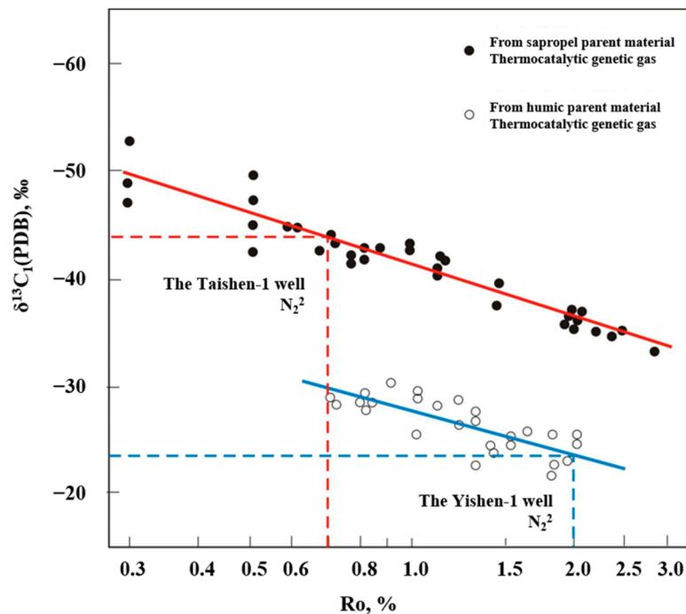
**Figure 5.** The relationship between the  $\delta^{13}C_1$  of  $N_2^2$  natural gas and  $R_o$  of its parent rock encountered by the Taishen-1 and Yishen-1 wells.
