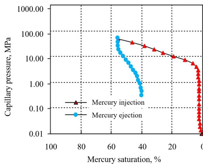
**Figure 6.** Capillary pressure curve of the Tertiary gray siltstone in the Taishen-1 well. (Depth: 3896.5 m,  $N_2^2$ ).
