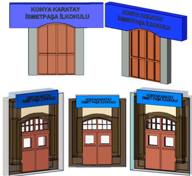
Figure 13. The final version of the created door (front and back) object saved in the family library.
