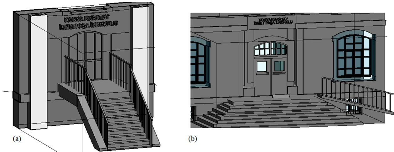
**Figure 15.** Manual drawing of stairs, ramps, and railing objects. (a) stairs and railing details and (b) entry ramp and staircase object.
