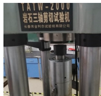
Figure 8. Test equipment (Rock triaxial shear testing machine produced by Changchun Jinlier Testing Machine Co.).
