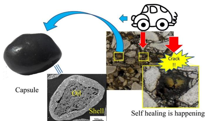
**Figure 4.** Characterization and healing process of saturated porous aggregates encapsulate rejuvenators [87].
