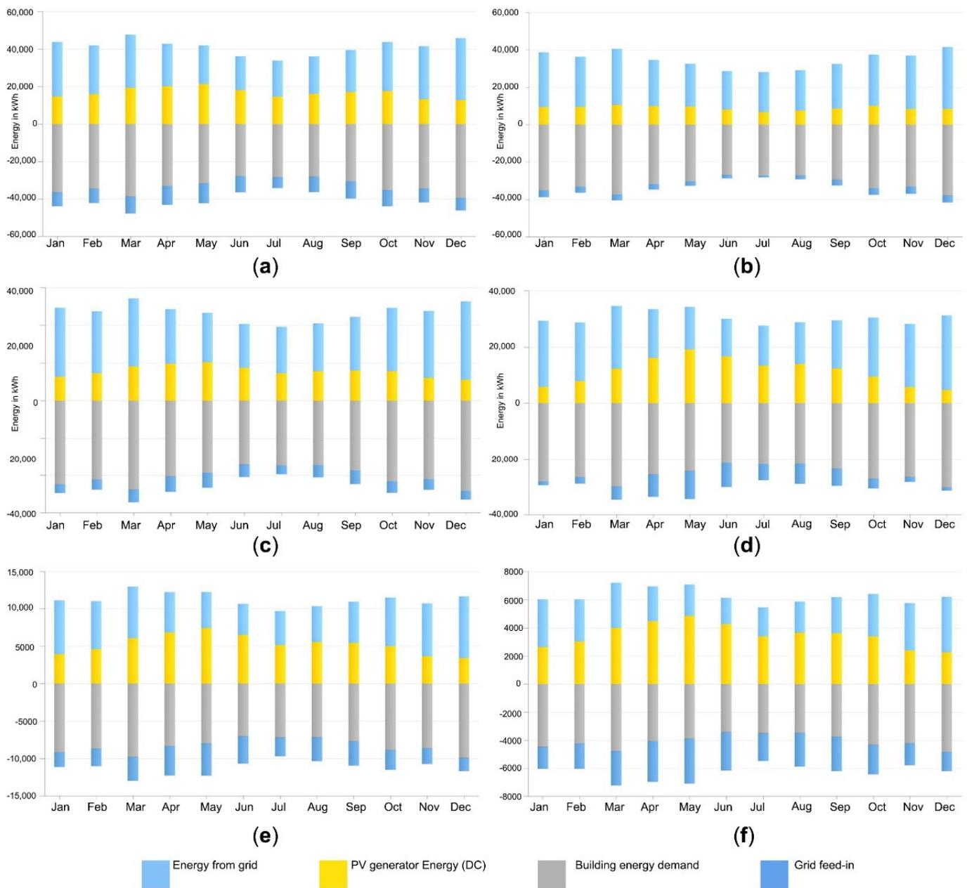
**Figure 8.** PV\*SOL energy simulation results for four apartment clusters (a–d), mixed-use (e), and multi-unit residential (f) buildings.
