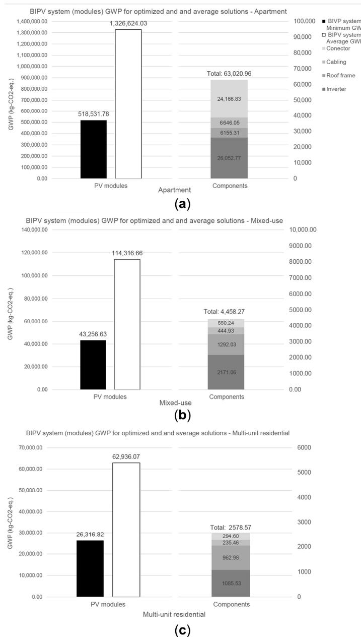
**Figure 6.** LCA results for the minimum and average GWP of BIPV modules (minimum and average system GWP) and BIPV system components for the (a) apartment, (b) mixed-use, and (c) multi-unit residential buildings.
