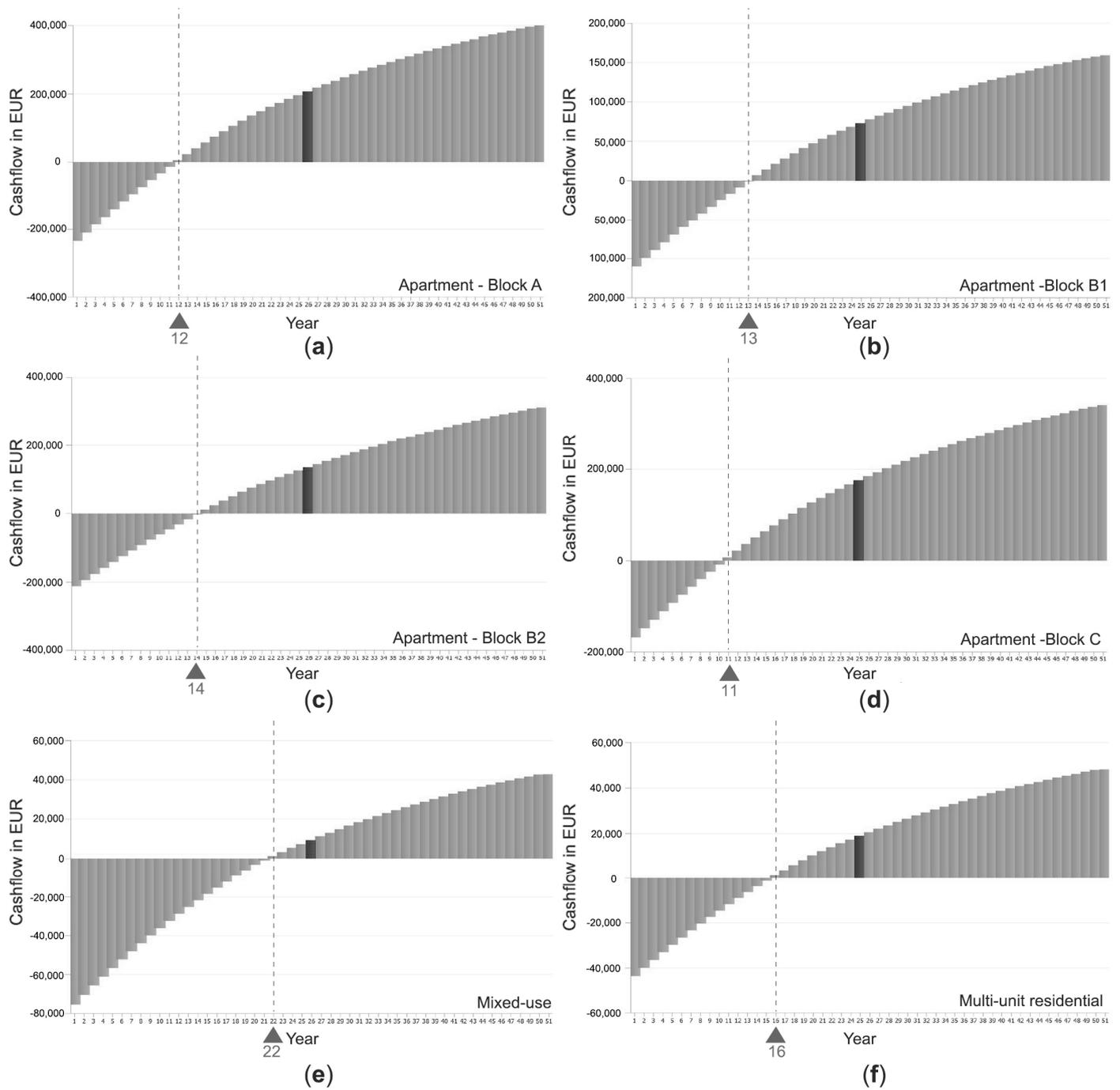
**Figure 9.** US NREL-based costing scenario NPV for the service life period of four apartment clusters (a–d), mixed-use (e), and multi-unit residential (f) buildings. Darker markings indicate discounted cash flow at 25 years of service life.
