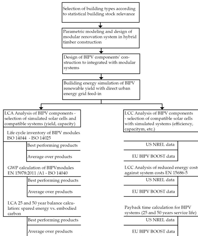
**Figure 1.** Methodological flowchart describing the execution of the research and the required calculations and standards involved in the simulation of renewable energy produced by BIPV systems and LCA/LCC. For LCA/LCC have been utilized multiple standards, such as ISO 14044 [40], ISO 14025 [41], ISO 14040 [42], EN ISO 15686-5 [43].
