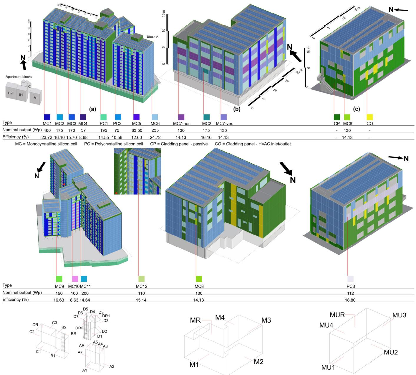
**Figure 5.** BIPV module design system for (a) an apartment building, (b) a mixed-use building, and (c) a multi-unit residential building with indication of module types (ID in Table A2) and technical specifications, indicated by specific color codes for the different selected PV module types.
