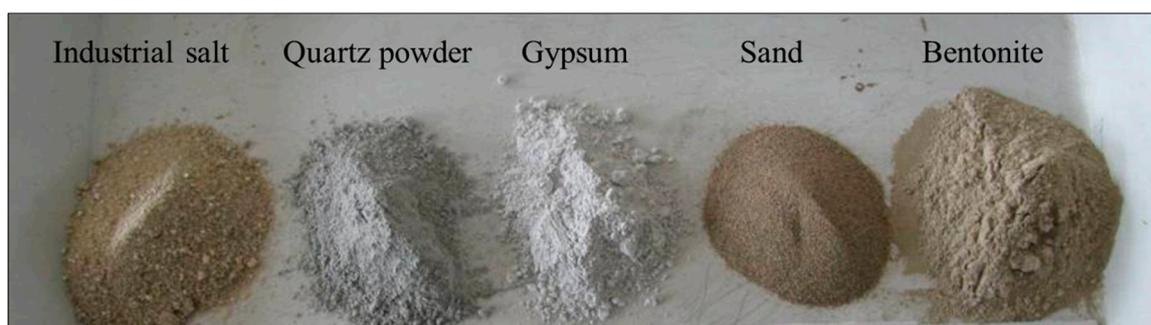
**Figure 1.** Materials of synthetic collapsible loess.
