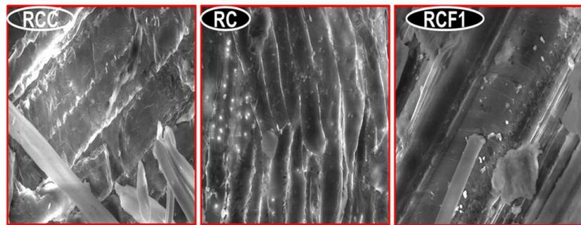
**Figure 3.** SEM images of the rice straw: RCC is control untreated sample, RC is 5% NaOH-treated sample, and RCF1 represents filtered sample of recycled NaOH treated with magnification of 1000 $\times$  times.
