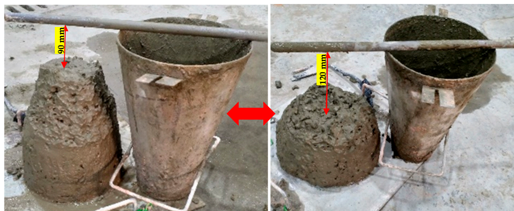
Figure 5. Typical concrete slump range for all N, H, and U concrete mixes.
